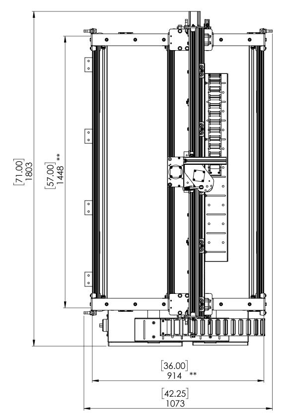
\*\*Dimension to outside edges of extrusion, use this measurement if building your own leg assembly
