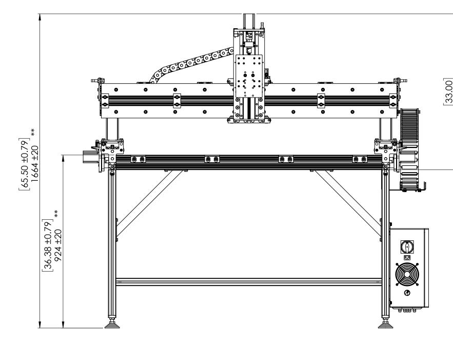
12" Travel Z-Axis will add 100mm (3.94") to top of machine \*\*Adjustment of leveling feet in leg kit will impact actual height dimension
