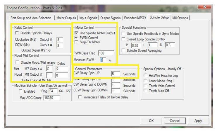
Under the "Spindle Setup" tab make the following changes:
