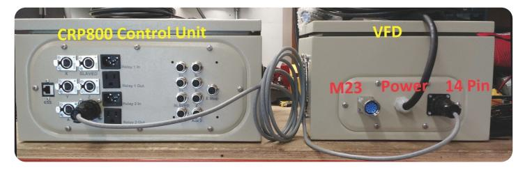
The included M23 cable should be used to connect your VFD to your spindle and the VFD power cable should be plugged into an appropriate L6-30 240 volt outlet.
