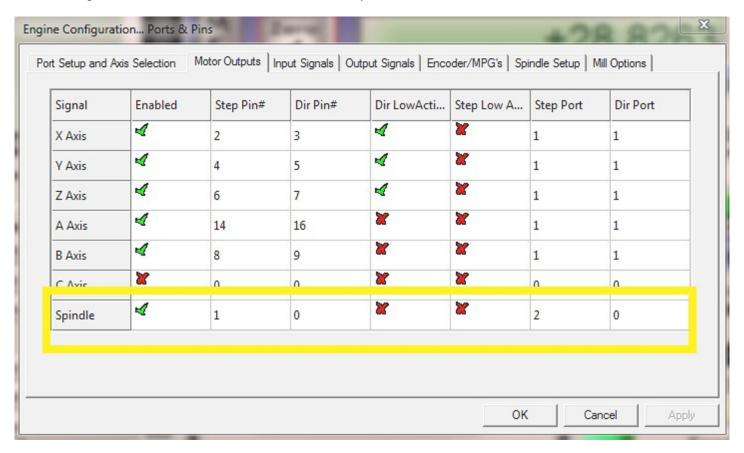
Under the "Motor Outputs" tab, make the following changes to the "Spindle" row:
