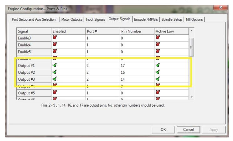
Under the "Output Signals" tab make the following changes:
