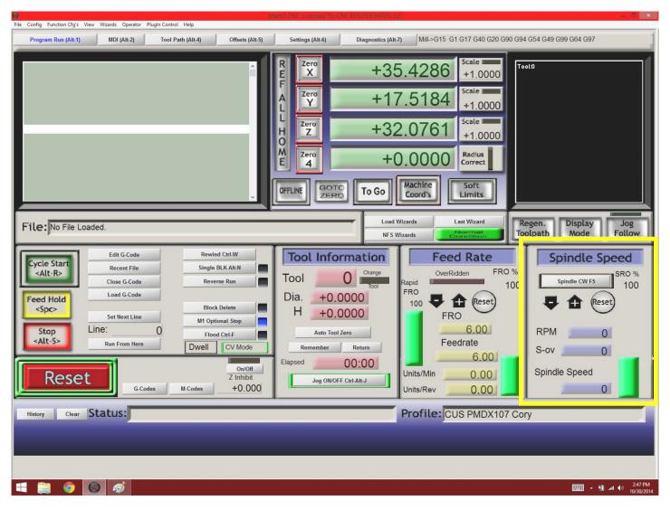
When using your spindle, enter a speed between 8000 and 24000 into the "**Spindle Speed**" box. If you enter a value too low, it will bump to 7980, too high and it will bump to 24000. If you accidentally enter a value too low or high, hit reset twice to clear the "Status."
