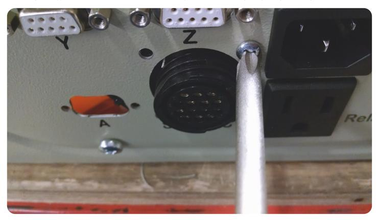
The 14 pin connector must now be wired to the break out board inside of the Control Unit. Install the four pin SUPU connector onto the break out board in the orientation and position shown.
