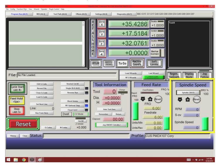
When using your spindle, enter a speed between 8000 and 24000 into the "**Spindle Speed**" box. If you enter a value too low, it will bump to 7980, too high and it will bump to 24000. If you accidentally enter a value too low or high, hit reset twice to clear the "Status."
