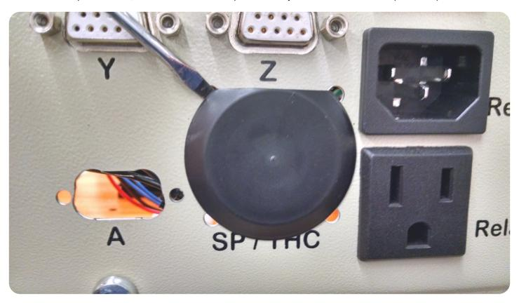
Next install the 14 pin connector from the back side of the gland plate, with the square plastic flange on the inside of the Control Unit. (See Below)
