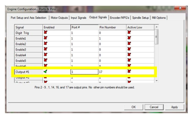
Again under "Ports and Pins" navigate to the "Output Signals" tab. Enable Output 1. The Output 1 Port and Pin numbers should be changed to 1 and 17, respectively.
