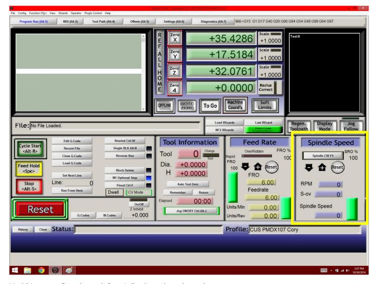
Mach3 is now configured properly for spindle relay and speed control.
