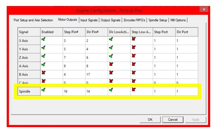
Select "Ports and Pins" from the "Config" drop down menu then navigate to the "Motor Outputs" tab.
