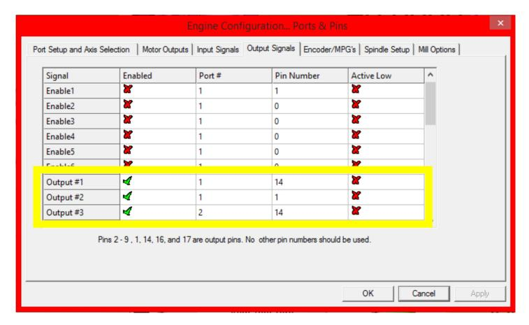
Again under "Ports and Pins" navigate to the "Output Signals" tab.
