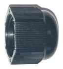
The left (as shown) threaded end of the strain relief should be installed into the gland plate of the control unit, from the exterior. The clamping collar (at left in photo) should then be threaded onto the strain relief, from the interior, to hold it in place on the gland plate.
