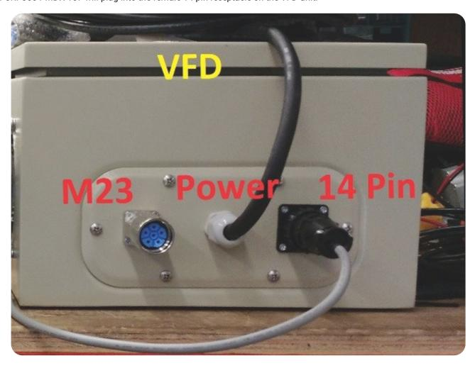
The included M23 cable should be used to connect your VFD to your spindle and the VFD power cable should be plugged into an appropriate L6-30 240 volt outlet.
