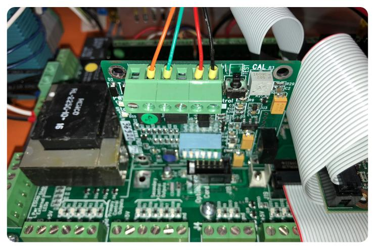
Insert the ferruled cable ends into the PMDX 107 isolated speed control card as shown. From left to right they will be:
