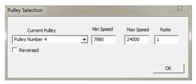
Under the drop down menu "Config" choose "Spindle Pulleys."
