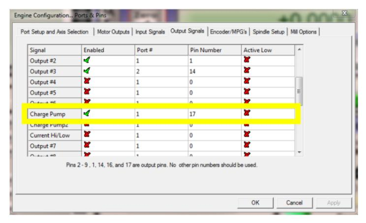
The "Charge Pump" Signal must be enabled, and its port and pin numbers should be 1 and 17, respectively.
