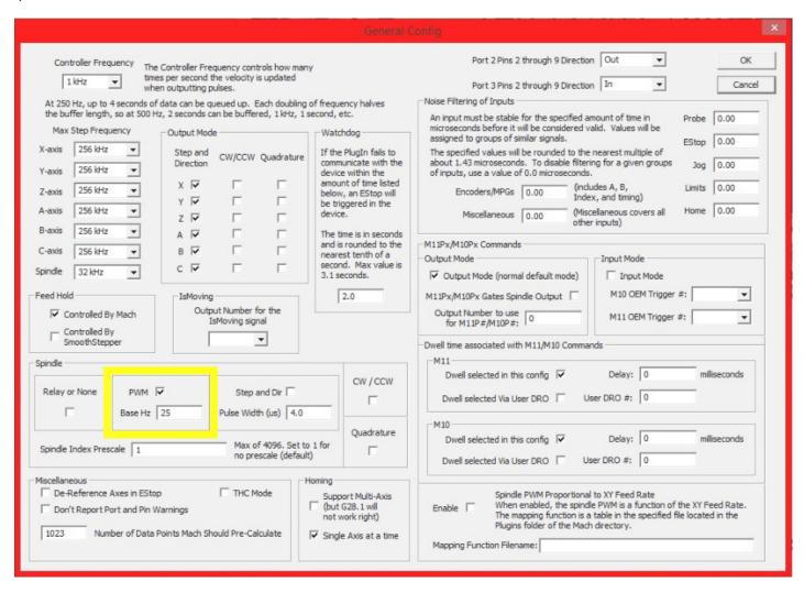
Under the Plugin Control drop down menu, select ESS-General Config and then make sure the PWM box is checked and the Base Hz is set to 25. Now Restart Mach3.
