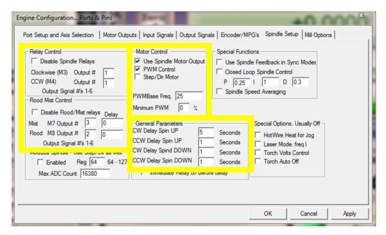
Again under "Ports and Pins" navigate to the "Spindle Setup" tab.
