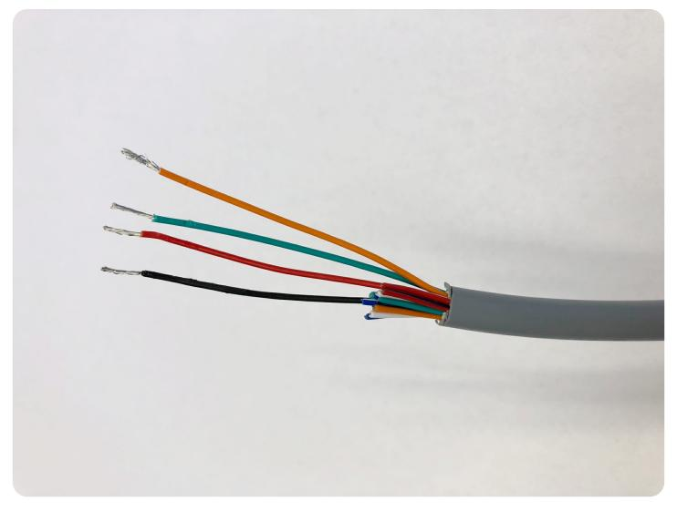
Separate out and strip the Black, Red, Orange, and Green wires. They may now be ferruled or tinned if you desire, although they will function as bare wires. The remaining wires are not used and can be cut back.
