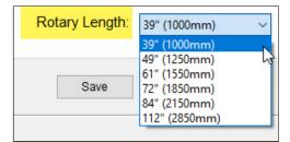
**Rotary Length:** If you selected an "Avid PRO CNC Rotary Axis" 4th Axis, you will have an option to specify the overall rotary length.
