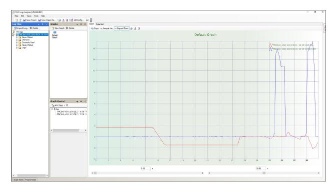
• **Default Graph** - By default the Tip Volts and Z Axis motion of the imported log file will be graphed on the right side of the application window.
