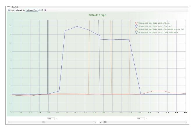
• **Changing the Graph Scale** - The sliders at the bottom of the graph will change the time scale of the graph and the position of the graph along said time scale. Shorten the timescale (right slider) and scroll across the graph (left slider) to the point during the cut you wish to analyze.
