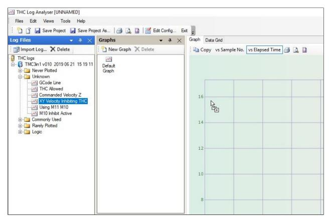
• Adding Log Data to the Graph - Expanding the THC log menu on the left of the screen will display the different data which can plotted and compared. To plot specific data, select it on the left of the screen then click, drag, and drop the data onto the graph (right side of the screen).
