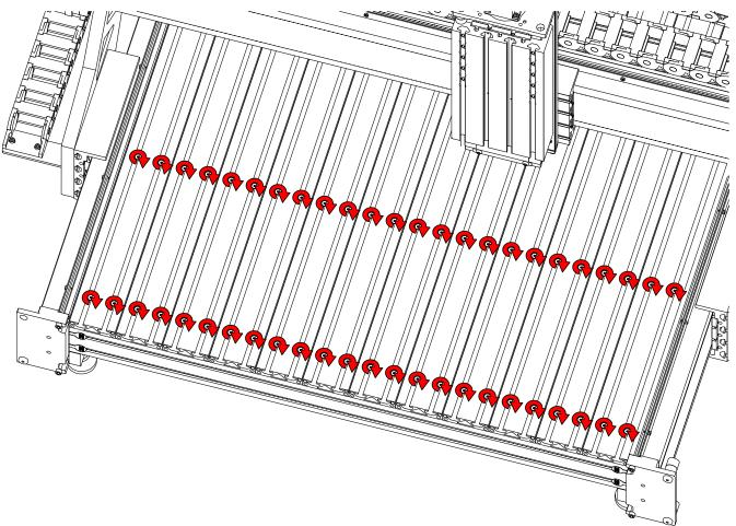
• Fully tighten the tabletop extrusion fasteners.
