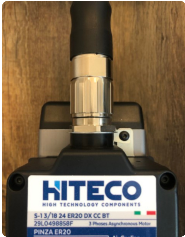
M23 Cable Fully Tightened
