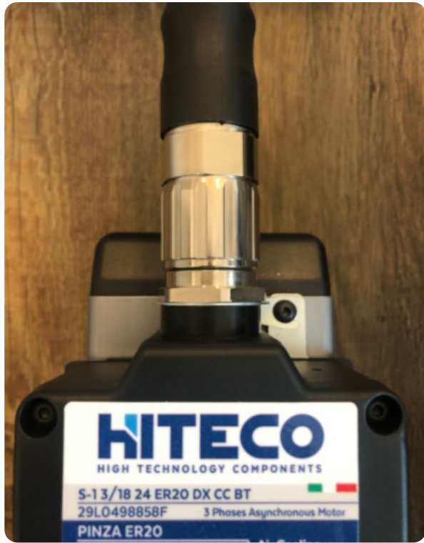
M23 Cable Fully Tightened
