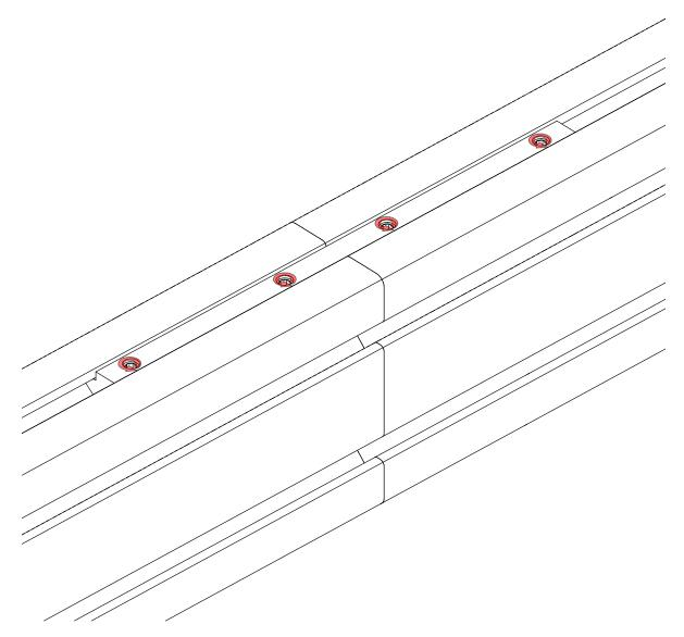
• Tighten the set screws in both splice bars.
