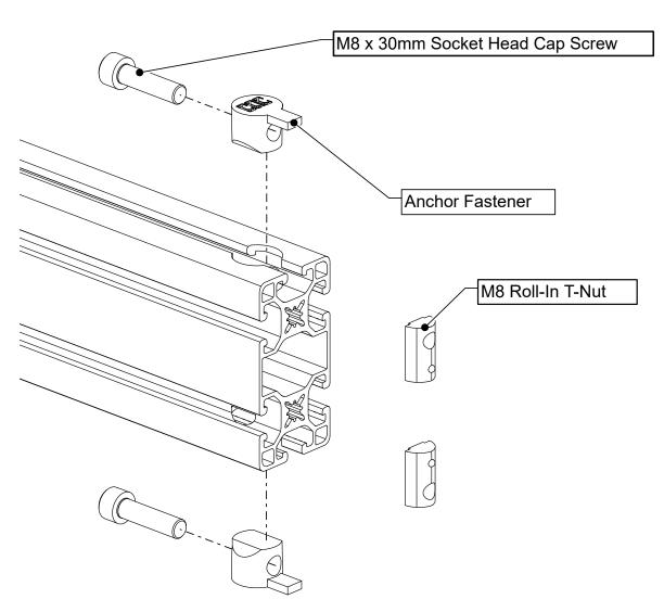
• Slide anchor fasteners into the two new pieces of leg extrusion.
