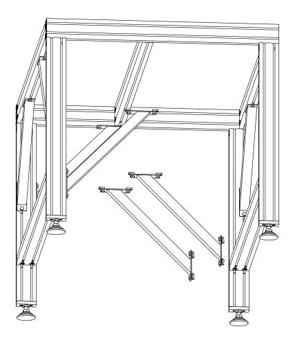
• Remove the leg gussets from both of the legs on the back of the machine.
