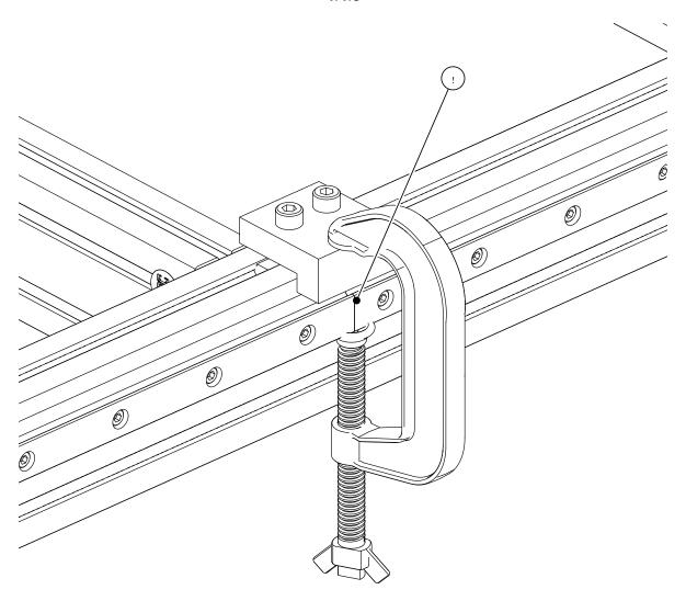
• Ensure the rails are flush at the splice.
