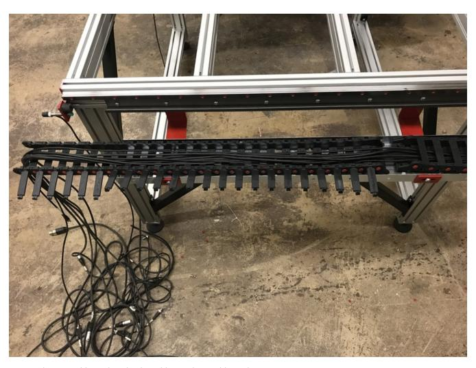
• Lay the new cable track under the cables on the Y cable track tray.
