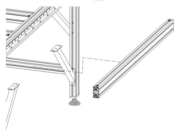
• Repeat the previous steps on the other side of the electronics mounting bar and remove the electronics mounting bar from the leg kit.
