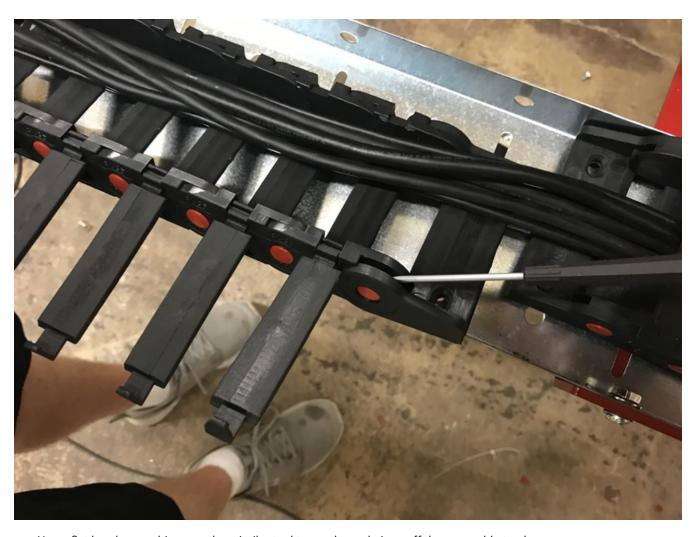
• Use a flat head screwdriver or other similar tool to pry the end piece off the new cable track.
