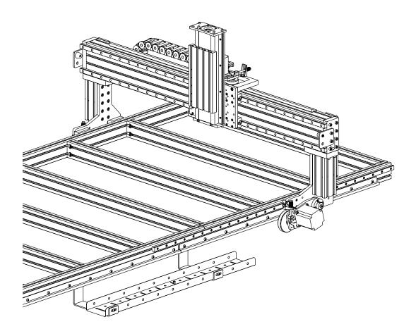
• Slide previously loosened rails down to the end of the newly added extrusion.
