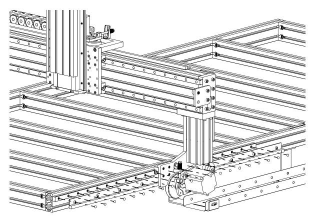
• Remove the plastic screw covers from the linear rails on both sides of the table.
