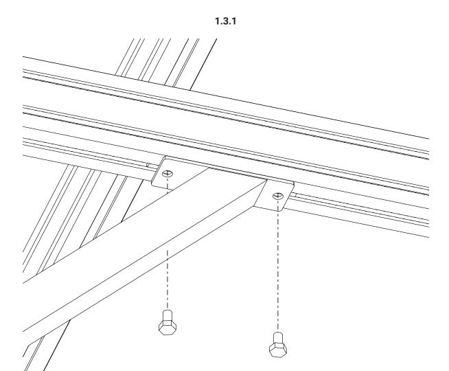
• Remove the indicated bolts from the electronics mounting bar.
