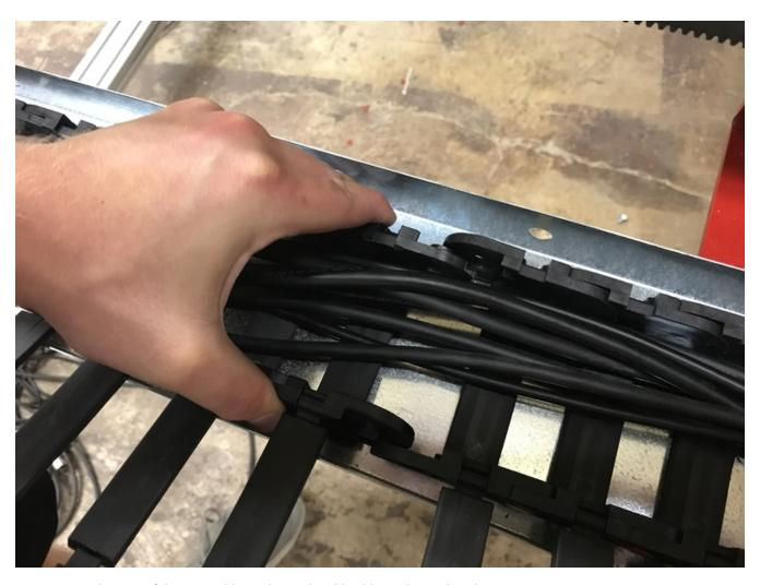
• Squeeze the new of the new cable track into the old cable track to splice the sections.
