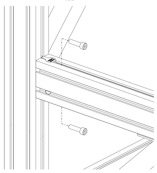
• Remove the indicated screws and anchor fasteners from the electronics mounting bar.
