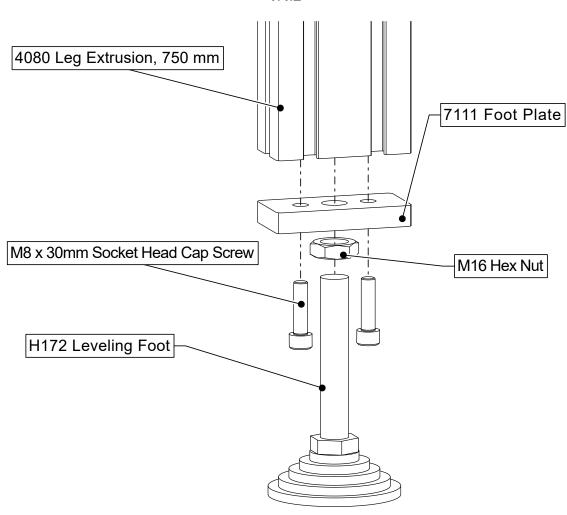
• Install foot assemblies onto the new legs
