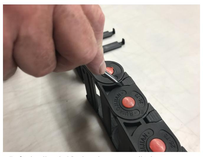
• Use a flat end screwdriver or other similar tool to open the covers on your new cable track.
