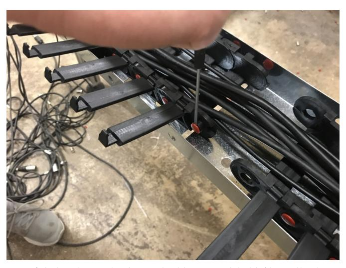
• Use a flat head screwdriver or similar tool to remove the red plastic covers on the last link of the new cable track
