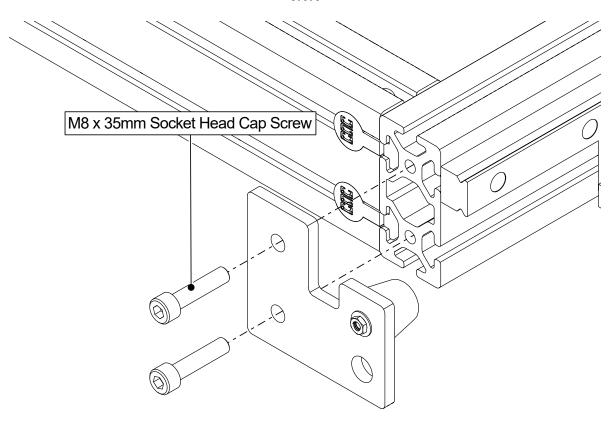
• Remove the bumpers from the front of the machine table.
