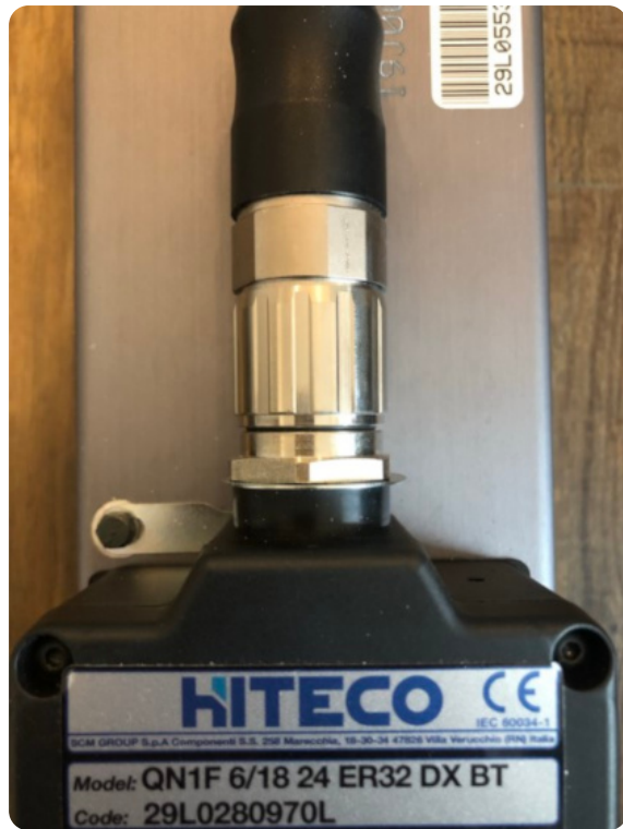
M23 Cable Fully Tightened
