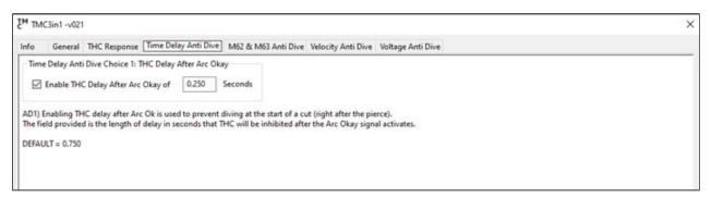
These anti-dive settings are the same as the THC main screen THC Anti-Dive tab. Changes made in the TMC3in1 plugin menu will be saved as default and overwrite defaults set by the THC main screen "Save as Default Anti-Dive Settings" button.
