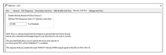
These anti-dive settings are the same as the main screen THC Anti-Dive tab. Changes made in the TMC3in1 plugin menu will be saved as default and overwrite defaults set by the THC main screen "Save as Default Anti-Dive Settings" button.
