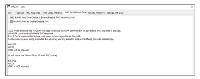
When enabled, the TMC3in1 will need to receive M62P4 commands in your GCode before THC response will be allowed. M63P4 commands can then be used to disable THC response. This type of anti-dive should not be disabled without consulting Avid CNC support.
