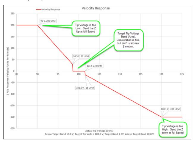
The above is a graphical representation of the THC motion (Z Axis Response Velocity - Y axis of graph) produced as a result of the incoming tip voltage signal from your plasma torch (Actual Tip Voltage - X Axis of graph). Reading the graph left to right, the data represents the following scenarios:
