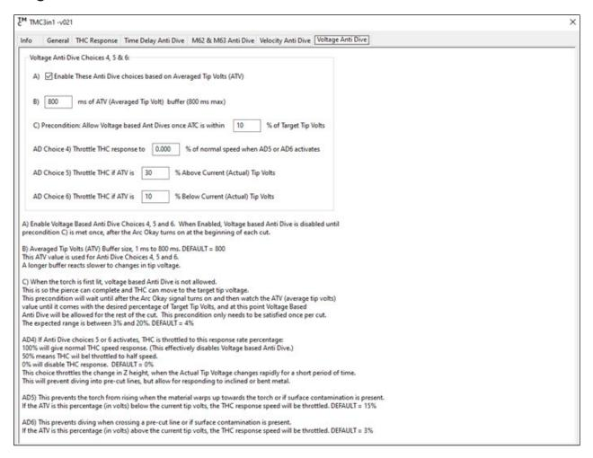
These anti-dive settings are the same as the main screen THC Anti-Dive tab. Changes made in the TMC3in1 plugin menu will be saved as default and overwrite defaults set by the THC main screen "Save as Default Anti-Dive Settings" button.
