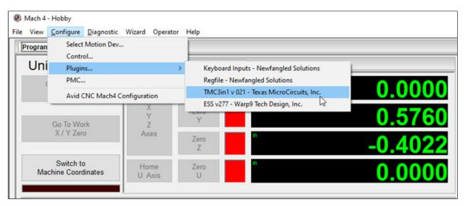
To access the TMC3in1 Plugin configuration navigate to TMC3in1 in the Plugins menu under the Configure pull down menu. *Any settings changes made from the TMC3in1 Plugin menu will be saved as defaults.*
