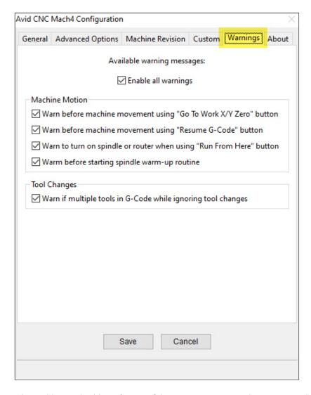
The Warnings tab allows the enabling or disabling of some of the warning messages that can occur during use of Mach4.
