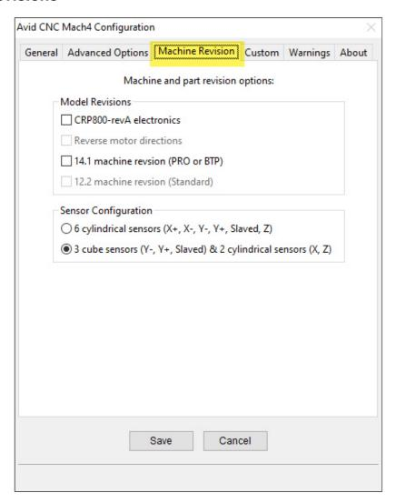
The Machine Revisions tab contains settings that apply for previous machine and electronics revisions.
