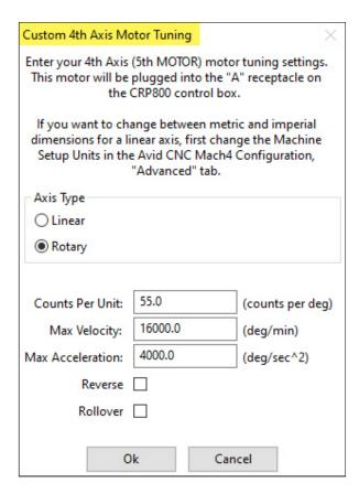
**Custom 4th Axis:** If you selected "Other" for the 4th Axis option, you will be able to specify the parameters listed below for motor tuning. If you want to use different units for motor tuning, first change the "Machine Setup Units" in the Advanced Settings tab.
