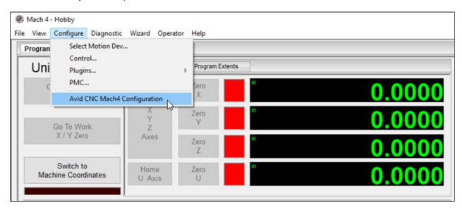
• Open the "Avid CNC Mach4 Configuration" window located in the Configure tab.
