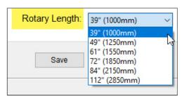
**Rotary Length:** If you selected an "Avid PRO CNC Rotary Axis" 4th Axis, you will have an option to specify the overall rotary length.
