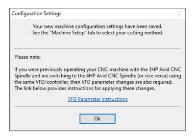
• If you had previously configured Mach4 with a 3 HP Avid CNC Spindle and are changing the **Spindle Type** selection to a 4 HP Avid CNC Spindle (or vice versa), you will see a notification letting you know that it is necessary to change VFD parameters. **This is only applicable if you are switching the spindle using the same VFD/controller.** Follow the link provided in the notification for instructions to make the necessary VFD parameter changes.
