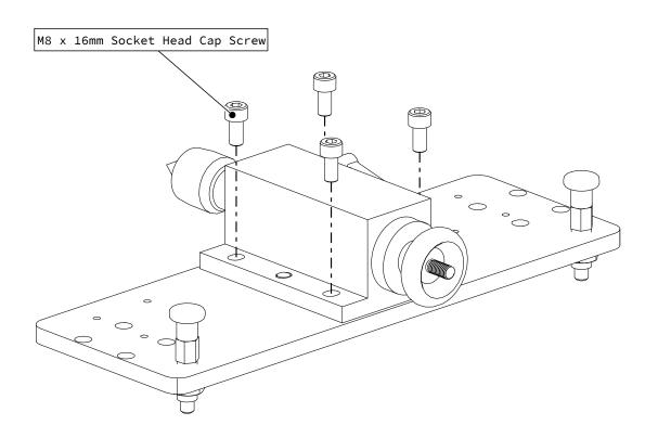
• Fasten the tailstock to the tailstock plate as indicated.
