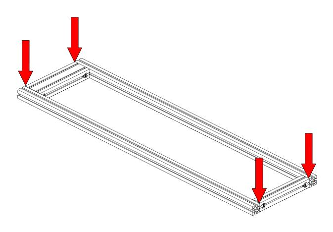
• Position the 4040 and 4080 extrusion assemblies flush with the ends of the rotary frame as indicated.
