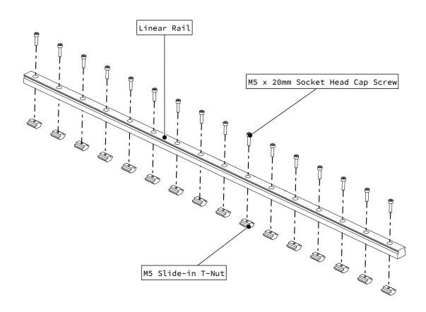
• Partially thread fasteners into the linear rail as indicated.
