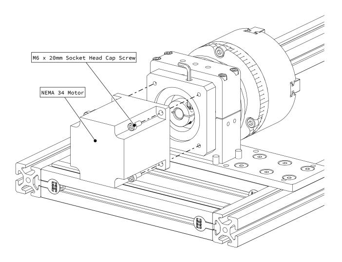
• Attach the motor to the reducer as indicated.
