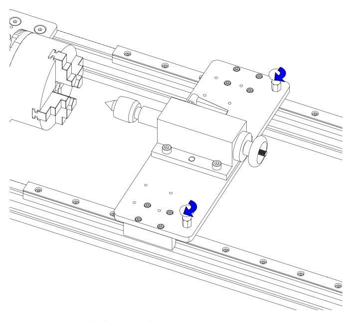
• Rotate the spring plunger handles to lock the tailstock in place.
