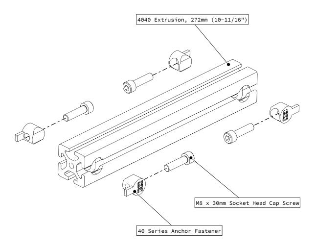
• Insert a socket head cap screw through the anchor fastener as indicated.
