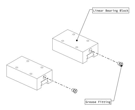
• Install grease fittings in the linear bearing blocks.
