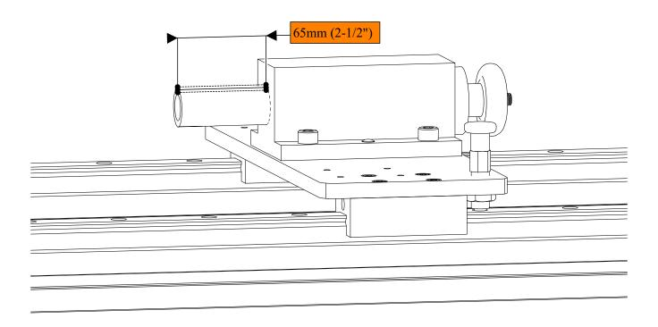
• Extend the tailstock 65mm (2-1/2") from the tailstock housing as indicated.
