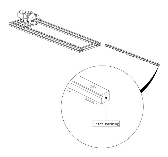
• Orient the second linear rail as indicated, with the marking facing away from the rotary frame.
