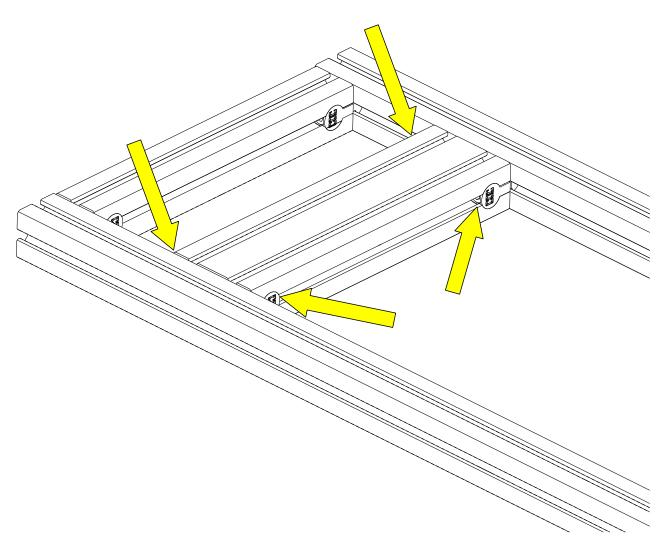
• Partially tighten the 4080 extrusion assembly anchor fasteners.
