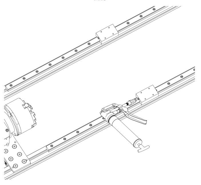
• Lubricate the linear bearing blocks with three pumps of grease per block.
