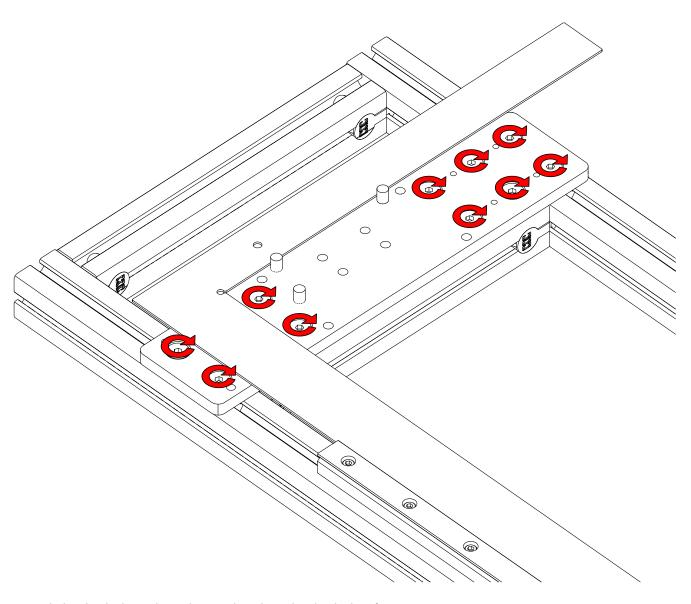
• With the chuck plate adjusted correctly, tighten the chuck plate fasteners.
