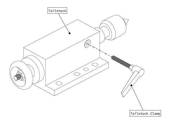
• Attach the tailstock clamp to the tailstock.
