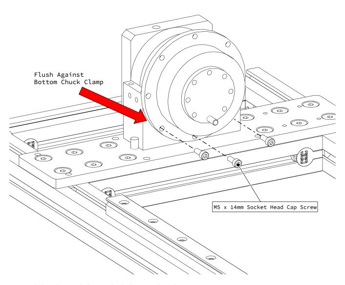
• Attach the reducer to the bottom chuck clamp as indicated.
