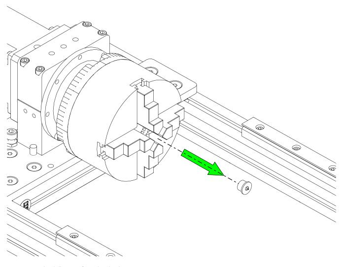
• Remove the drill center from the chuck.
