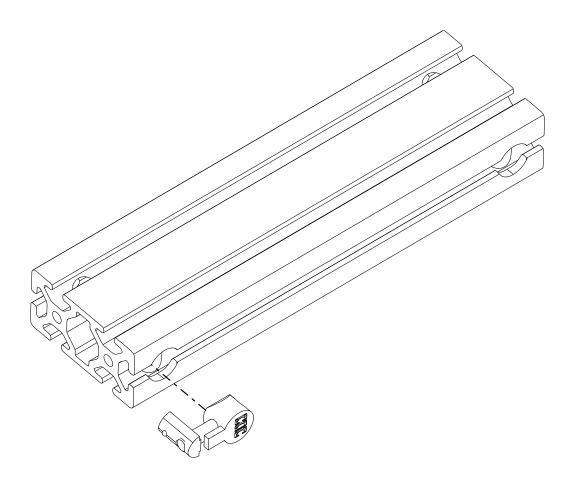
• Slide the anchor assembly into the 4080 extrusion.
