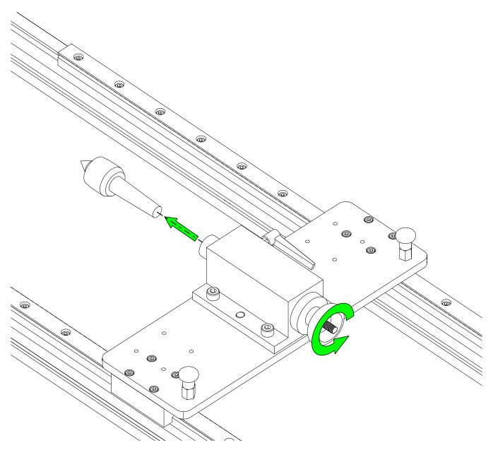
• Turn the tailstock handle counter-clockwise to remove the live center.
