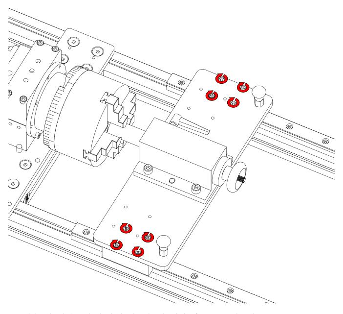
• With the tailstock clamped in the chuck, tighten the tailstock plate fasteners as indicated.
