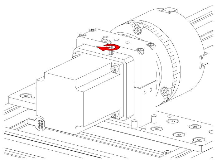
• Fully tighten the shaft collar using the 4mm allen wrench.
