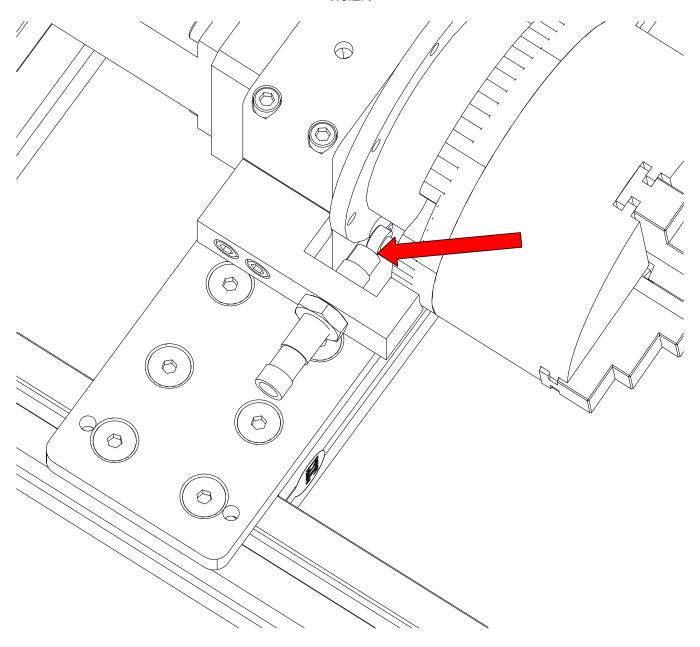
• Thread the sensor in until it touches the shoulder bolt.
