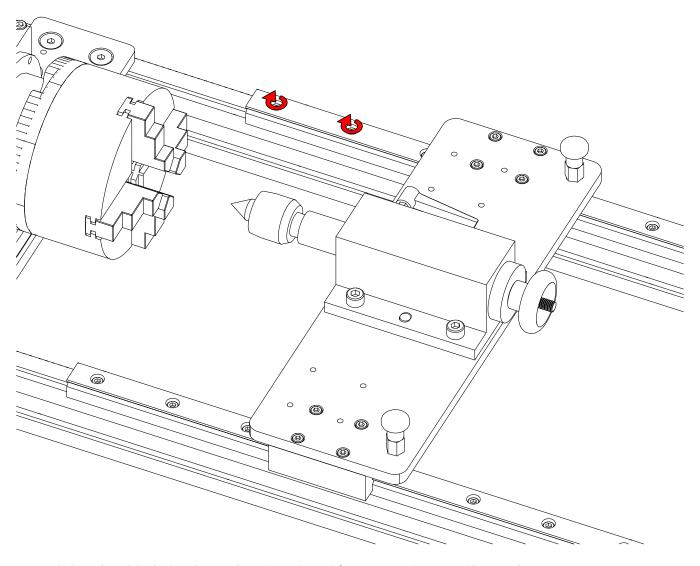
• With the tailstock locked in place, tighten the indicated fasteners on the second linear rail.
