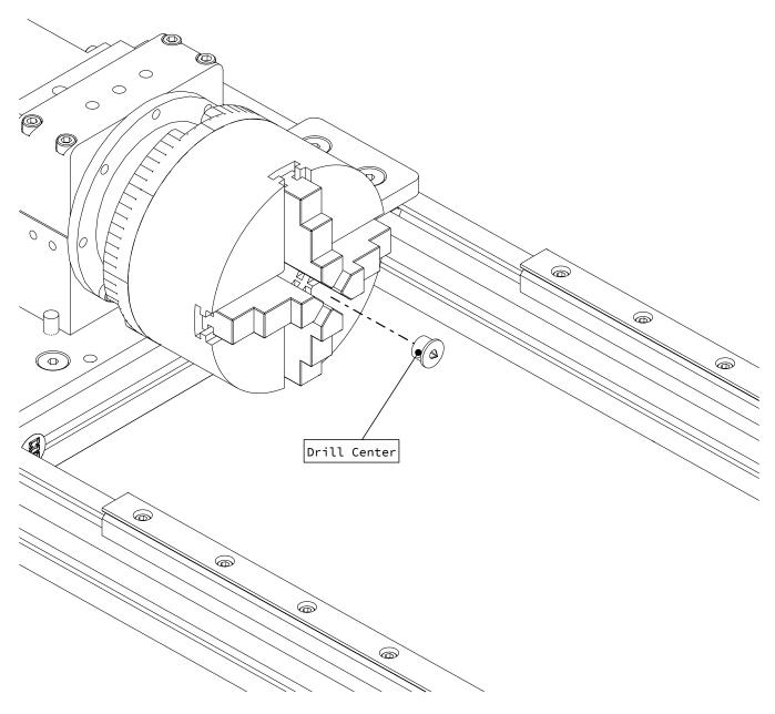
• Insert the drill center into the chuck as indicated.
