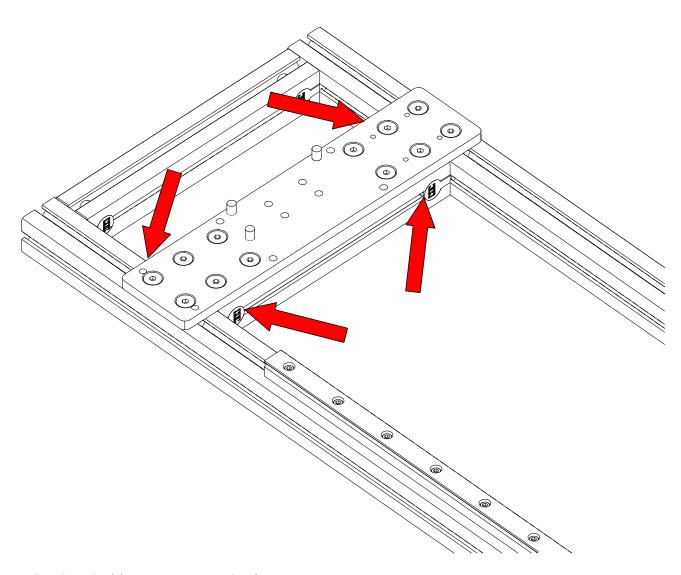
• Fully tighten the (4) 4080 extrusion anchor fasteners.
