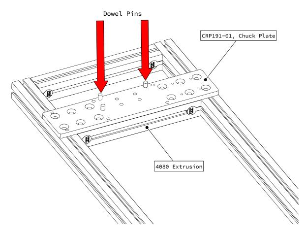
• Place the chuck plate on top of the 4080 extrusion as indicated.
