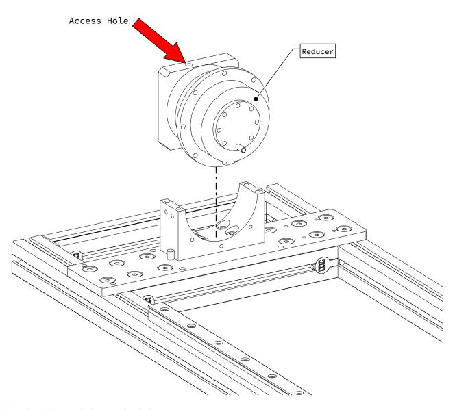
• Place the reducer in the bottom chuck clamp.
