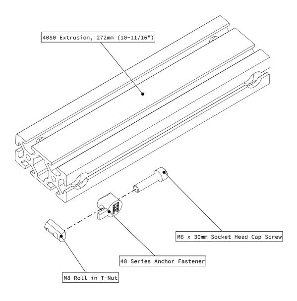
• Thread a socket head cap screw into the T-Nut through the anchor fasteners, as indicated.
