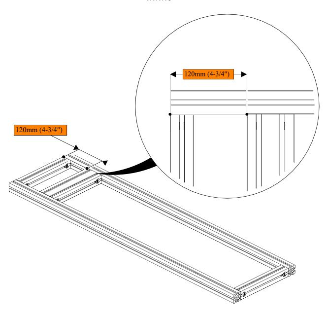
• Position the 4080 extrusion assembly 120mm (4-3/4") from the end of the rotary frame as indicated.
