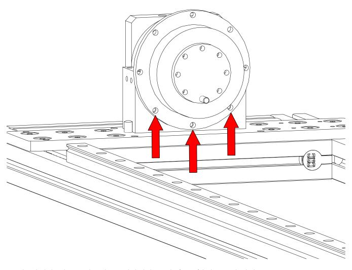
• Align the holes shown in the reducer with the holes on the front of the bottom chuck clamp.
