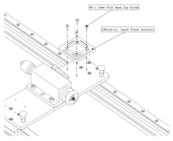
• Attach the touch plate isolator to the tailstock plate as indicated.
