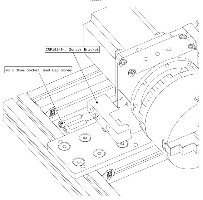
• Attach the sensor bracket to the bottom chuck clamp as indicated.
