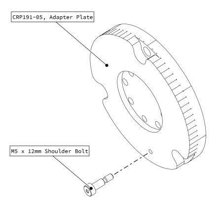
• Attach the M5 shoulder bolt to the adapter plate as indicated.
