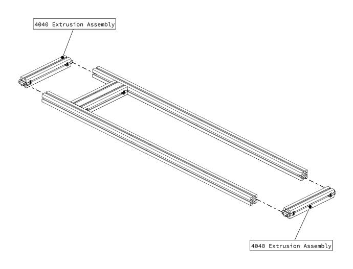
• Slide a 4040 extrusion assembly into the rotary frame on each end as indicated.
