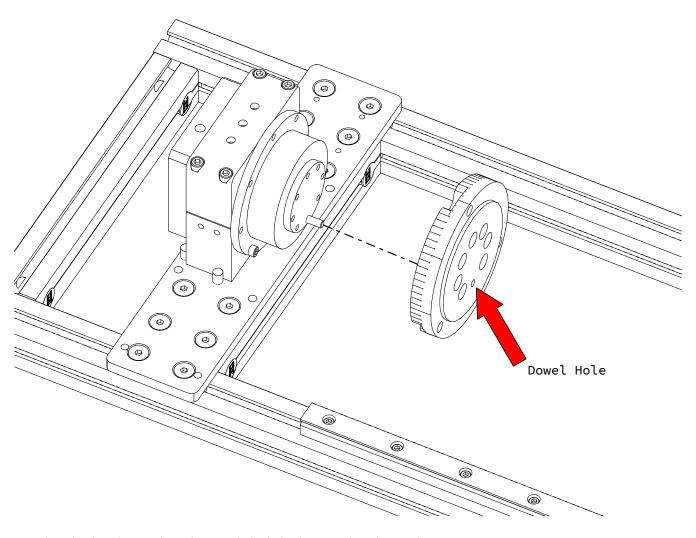
• Align the dowel pin in the reducer with the hole shown in the adapter plate.
