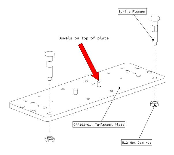
· Attach spring plungers to the tailstock plate as indicated.
