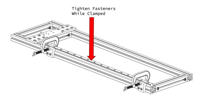
• Tighten the rail fasteners while clamped.
