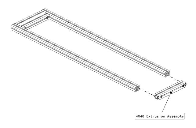
• Slide the 4040 extrusion assembly into the rotary frame as indicated.
