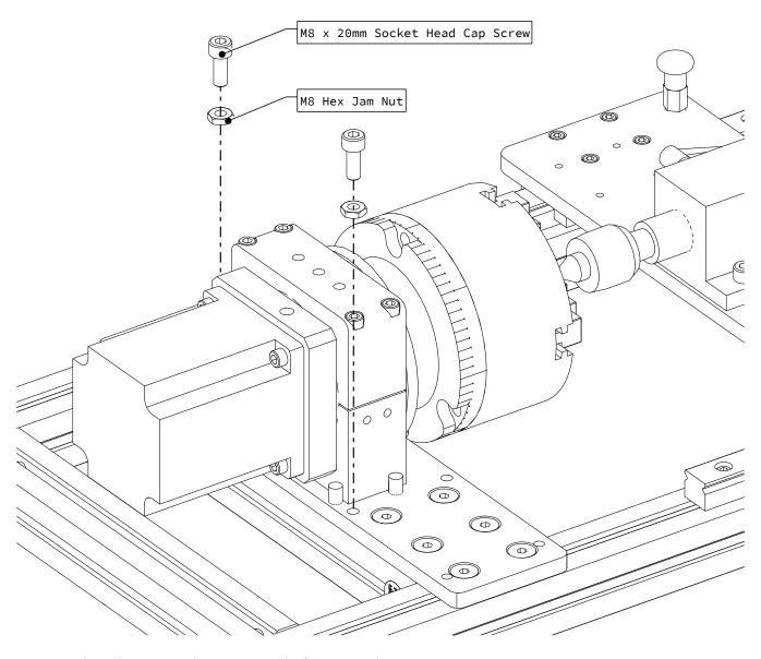
• Insert the jack screws and jam nuts into the front or rear locations.
