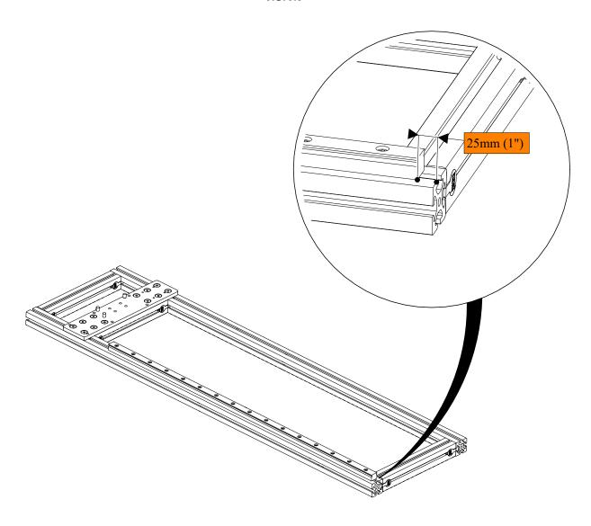
• Position the rail 25mm (1") from the end of the rotary frame as indicated.
