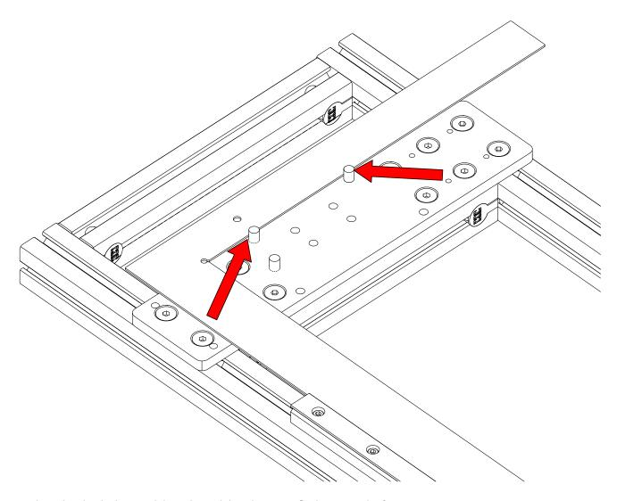
• Adjust the chuck plate until the indicated dowel pins are flush against the framing square.
