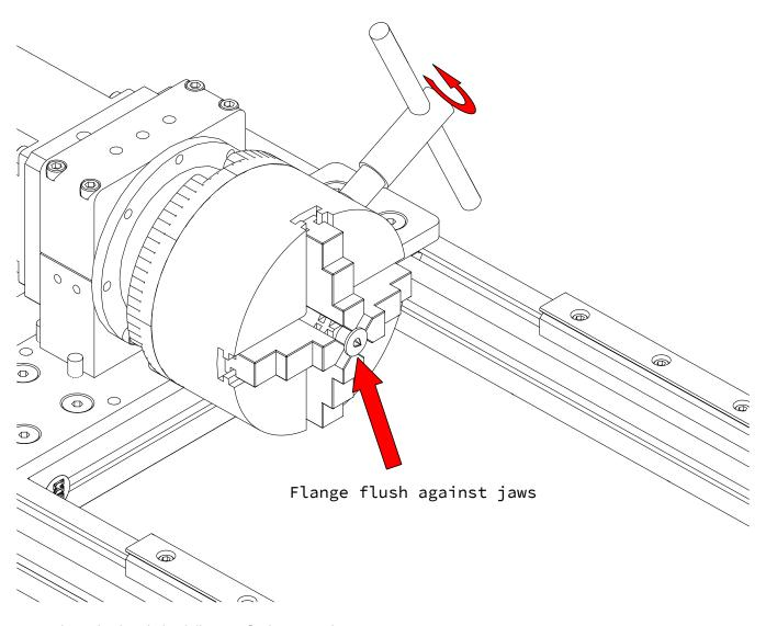
• Tighten chuck with the drill center flush against the jaws.
