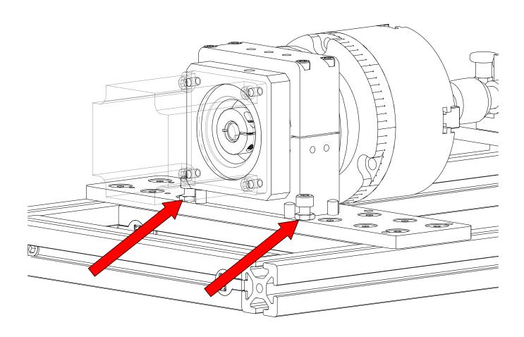
• Tighten the two jam nuts.
