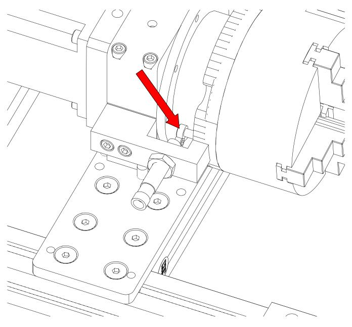
• Rotate the chuck to align the shoulder bolt with the sensor.
