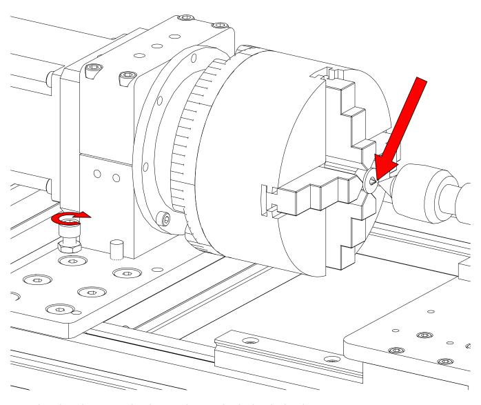
• Tighten the jack screws to align the points between the chuck and tailstock.
