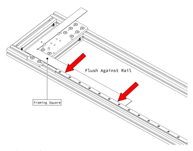
• Place a framing square flush against the linear rail as indicated.
