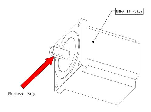
• Remove the motor key.
