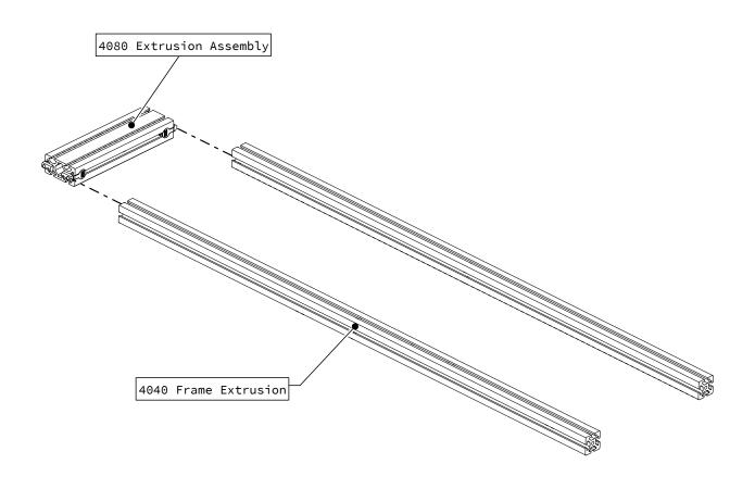
• Slide the 4080 extrusion assembly into the 4040 frame extrusion pieces as indicated.
