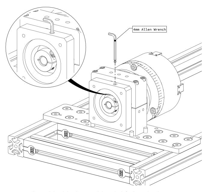
• Insert a 4mm allen wrench through the reducer access hole, into the shaft collar as indicated.
