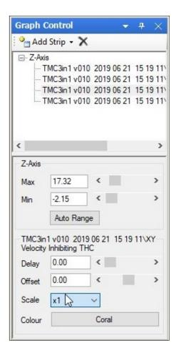
• Scaling Log Data - The Graph Control menu allows you to change the scale of individual data. The original scale of different data (Z axis height 0-8in, Tip volts 100-200V) can be altered (scale x10 or scale /10) to make them more easily comparable.
