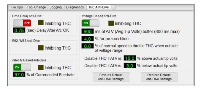
**Adjusting the THC settings** - The cut analyzed in the above example was successful, so the settings may not need adjustment. However, if an unsuccessful cut (crashed torch, low cut quality) is analyzed it may identify the fault with the THC settings causing the issue.
