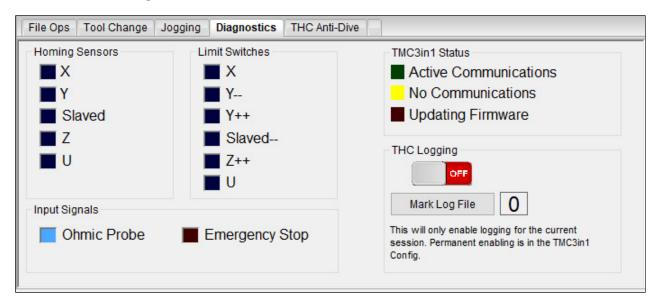
• Setting up THC logging in Mach4 - To collect THC Log data, ensure the THC Logging toggle is ON.
