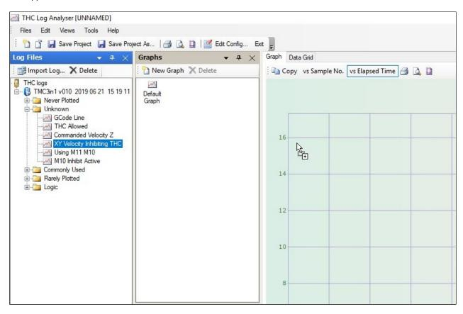
• Adding Log Data to the Graph - Expanding the THC log menu on the left of the screen will display the different data which can plotted and compared. To plot specific data, select it on the left of the screen then click, drag, and drop the
