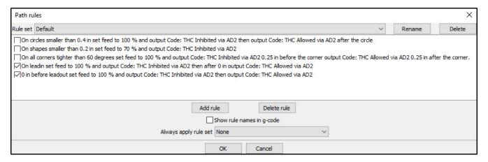
• The Path Rules window will then be displayed. The default rule set will have been installed by the "AvidCNC for SheetCam" installer. By default the only path rules which will be enabled turn THC motion off during lead in and lead out moves. To disable or enable path rules click the checkbox to the left of the path rule name.
