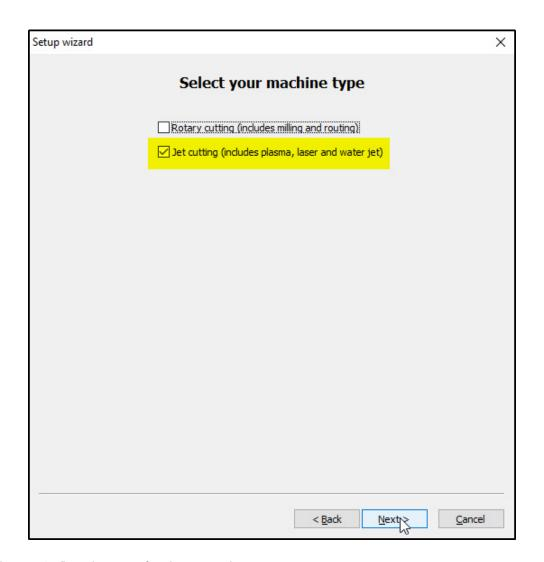
• Select "Jet cutting" machine type for plasma machines.
