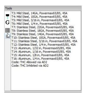
• To open the cutting rules editor press the Cut Rules button on the left of the Tools menu on the left of the SheetCam application window, or use the drop down menu Tools -> Cutting Rules.
