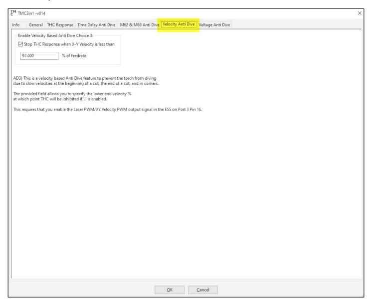
These anti-dive settings are the same as the main screen THC Anti-Dive tab. Changes made in the TMC3in1 plugin menu will be saved as default and overwrite defaults set by the THC main screen "Save as Default Anti-Dive Settings" button.
