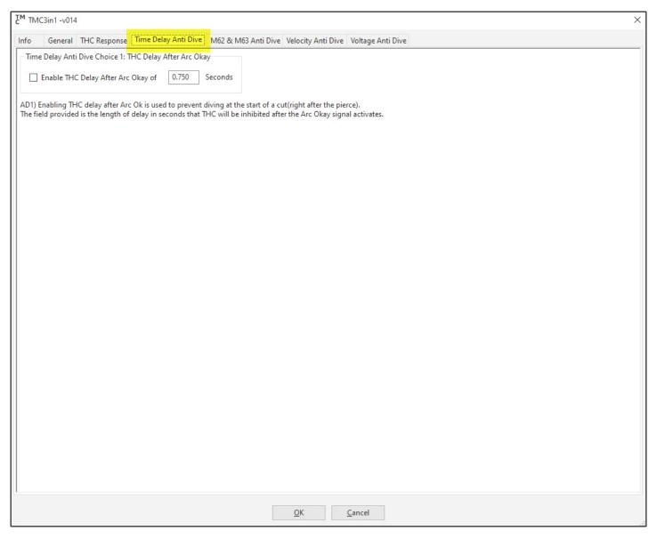
These anti-dive settings are the same as the THC main screen THC Anti-Dive tab. Changes made in the TMC3in1 plugin menu will be saved as default and overwrite defaults set by the THC main screen "Save as Default Anti-Dive Settings" button.
