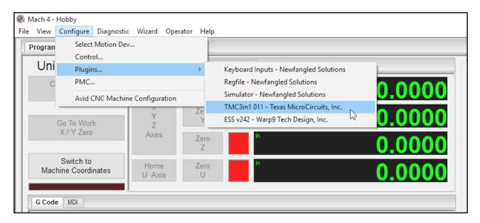
To access the TMC3in1 Plugin configuration navigate to TMC3in1 in the Plugins menu under the Configure pull down menu. *Any settings changes made from the TMC3in1 Plugin menu will be saved as defaults.*
