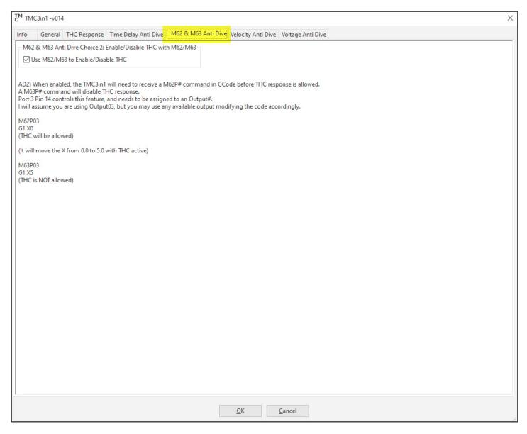
When enabled, the TMC3in1 will need to receive M62P4 commands in your GCode before THC response will be allowed. M63P4 commands can then be used to disable THC response. This type of anti-dive should not be disabled *without consulting Avid CNC support.*
