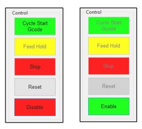
• **Collect Data** - Load G-Code of the cut you wish to log. Once your settings are properly configured for the plasma cutting operation click the "Disable" button on the bottom left of the Mach4 main screen (This will stop logging). When you are ready to cut, press the "Enable" button in the bottom left of the Mach4 main screen (This will start logging) and then "Cycle Start" to execute the cut. Once the cut is complete press "Disable" again (this will stop logging and save the log file).
