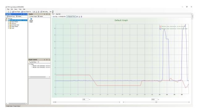
• **Default Graph** - By default the Tip Volts and Z Axis motion of the imported log file will be graphed on the right side of the application window.
