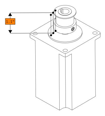
• Adjust the motor pulley such that the top of the pulley is 1.1" (28mm) from the motor flat.
