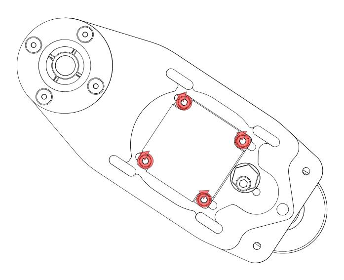
• Fully tighten the highlighted fasteners.
