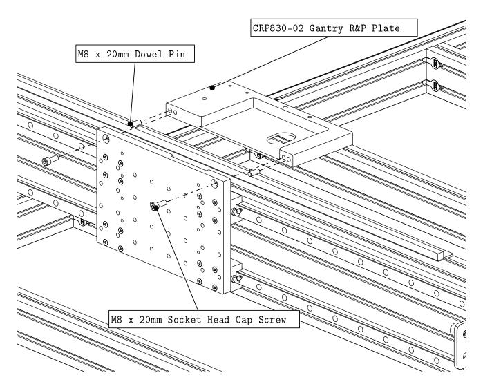
• Attach the Gantry R&P Plate to the Gantry Plate as indicated.
