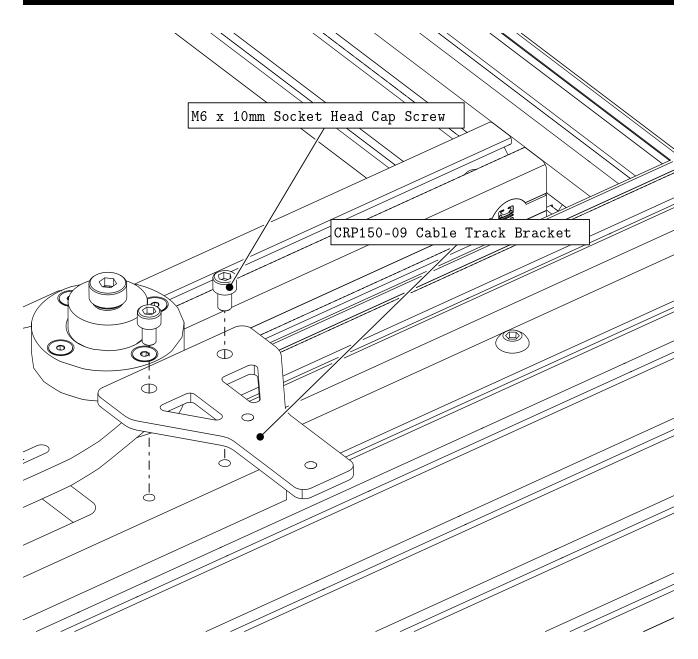
• Attach the gantry cable track bracket to the Gantry R&P Plate as indicated.
