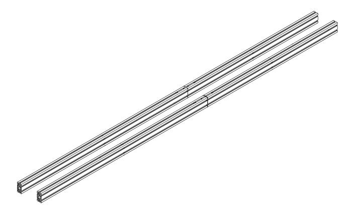
• Repeat the previous steps to form two spliced extrusion sections.
