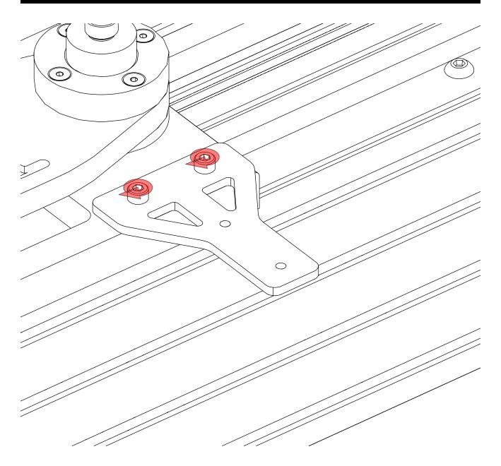
• Tighten the highlighted fasteners.
