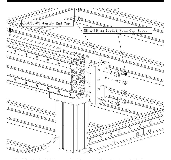
• Install a Gantry End Cap on the other end of the extrusion as indicated.
