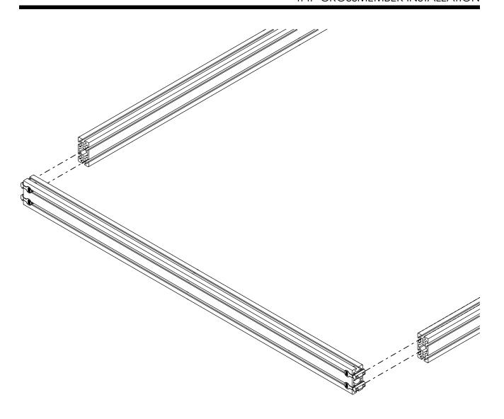
• Slide the t-nuts into the frame extrusion as indicated.
