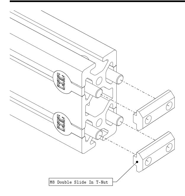
• Loosely thread the double t-nuts onto the socket head cap screws as indicated.
