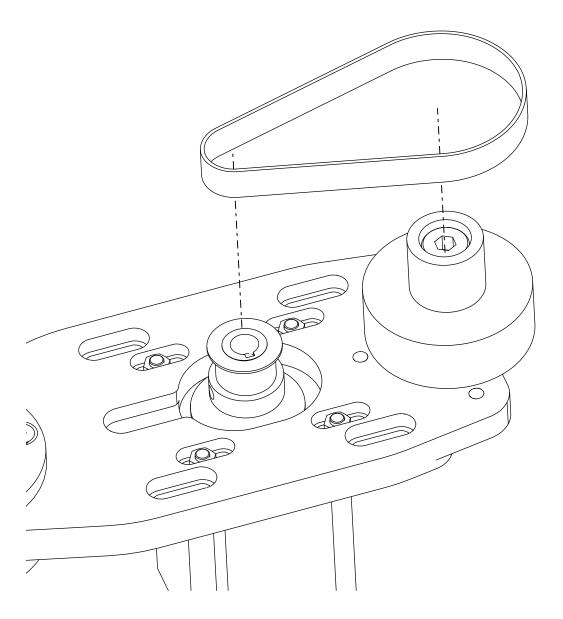
• Slide the drive belt around the motor pulley and drive spindle.
