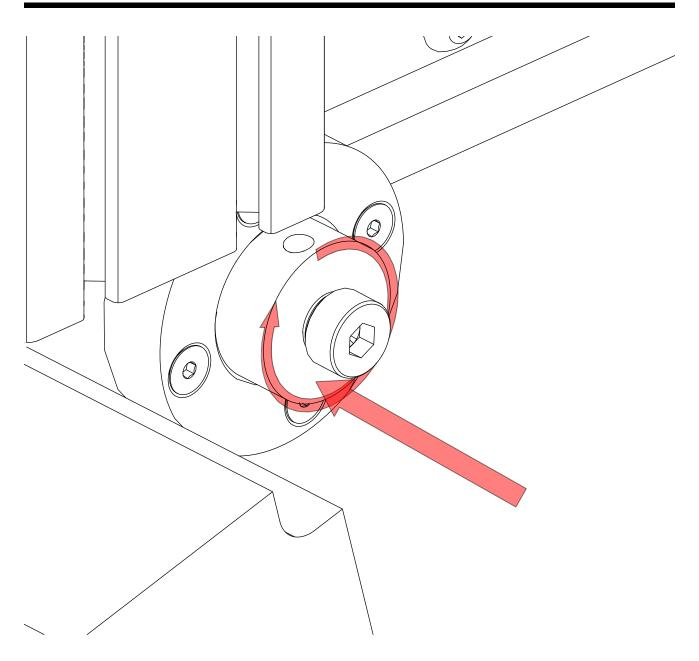
• While pushing in on the collar bearing eccentric, rotate it clockwise until the collar bearing starts rotating inside of the plate.
