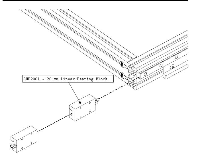
• Slide two linear bearing blocks onto a rail as pictured.
