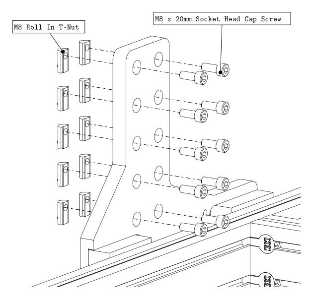
• Thread fasteners through the holes in the riser plate as indicated.
