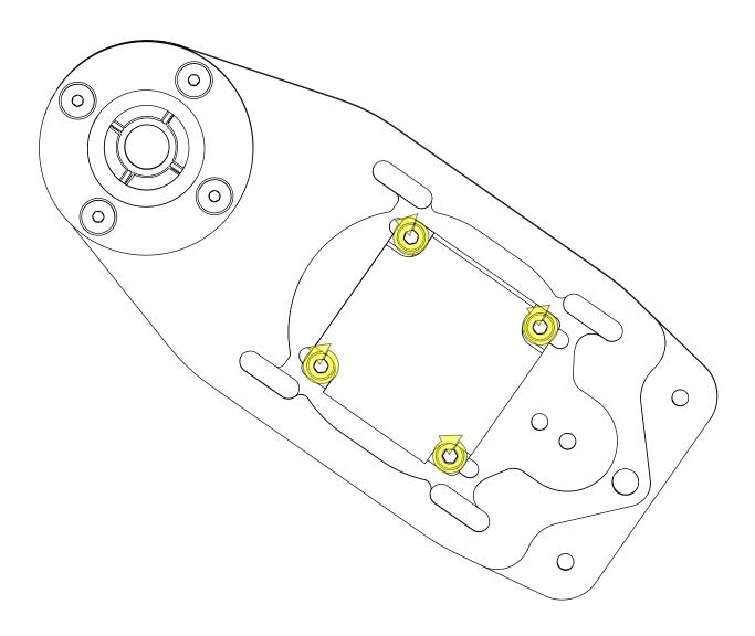
• Partially tighten the highlighted fasteners.
