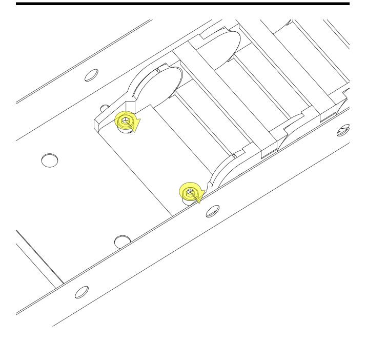
• Partially tighten the highlighted fasteners.
