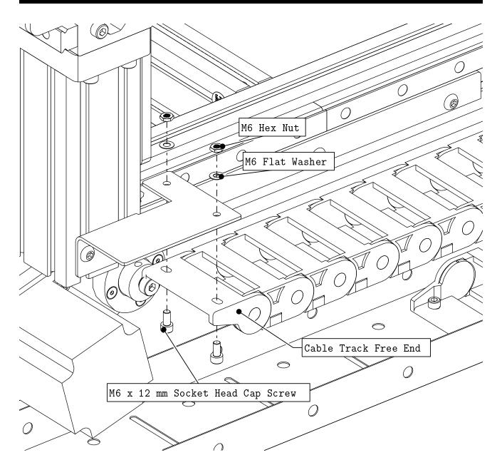
• Attach the remaining end of the cable track to the riser bracket as indicated.
