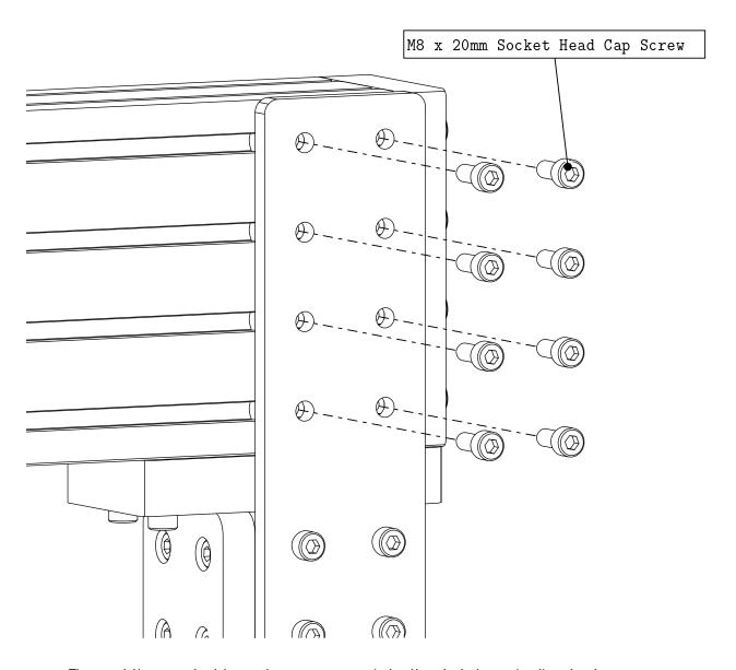
• Thread the socket head cap screws into the t-slots as indicated.
