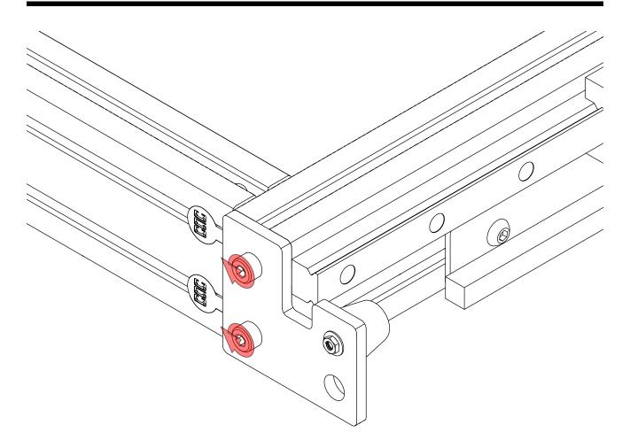
• Tighten the highlighted fasteners.
