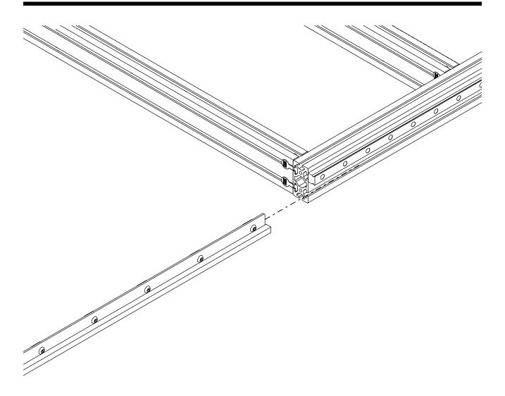
• Slide one of the sections of gear rack into the extrusion.
