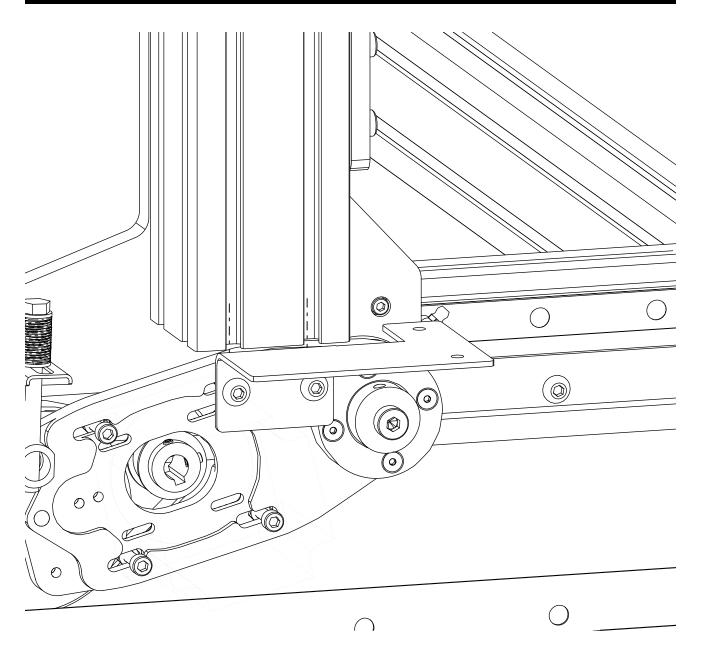
• Slide the riser cable track bracket into the riser extrusion.
