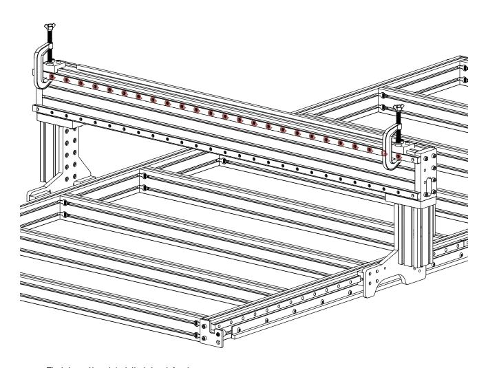
• Tighten the highlighted fasteners.
