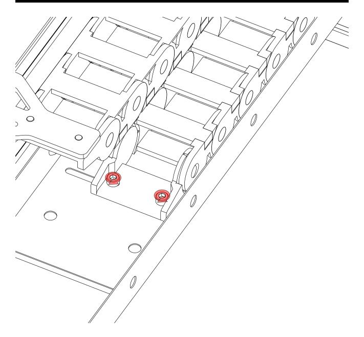
• Fully tighten the highlighted fasteners.
