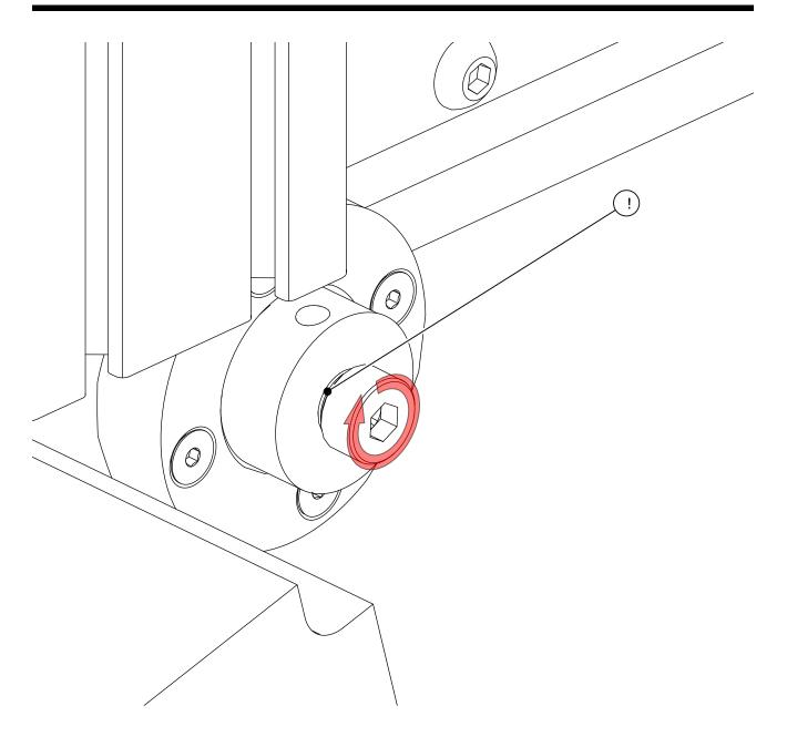
• Fully tighten the highlighted fastener.
