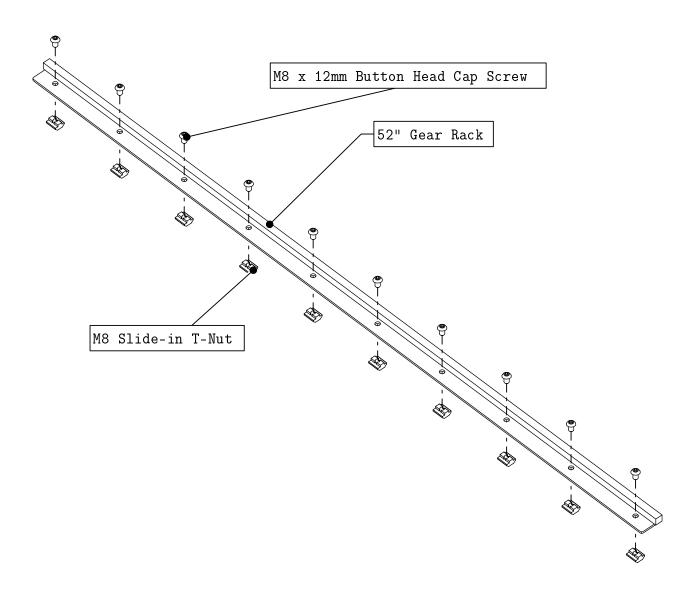
• Thread the indicated fasteners into the gear rack.
