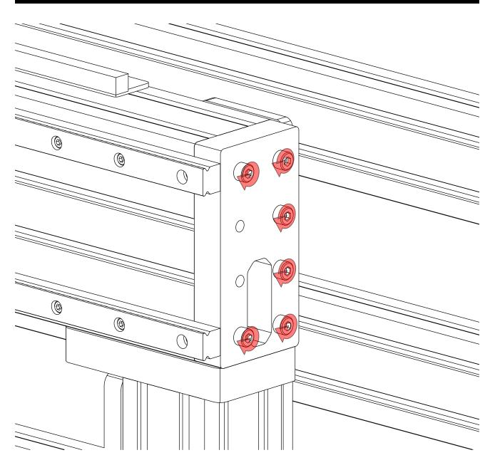
• Tighten the highlighted fasteners.
