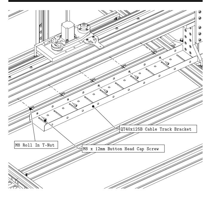
• Attach a cable track tray to the bottom t-slot of the gantry extrusion as indicated.
