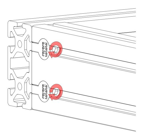
• Tighten the socket heads in each of the anchor assemblies to secure the frame.
