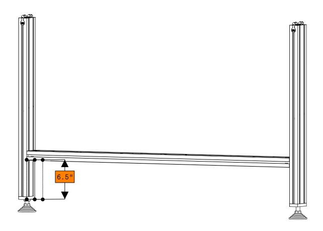
• Position the crossmember 6.5" (160mm) from the bottom of the leg.
