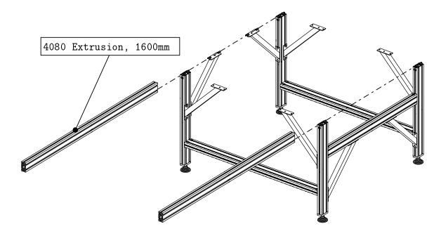
• Attach two of the leg assemblies to two 1600mm lengths of 4080 extrusion as indicated.
