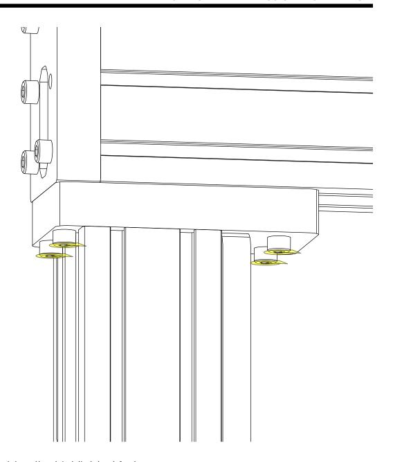
• Partially tighten the highlighted fasteners.
