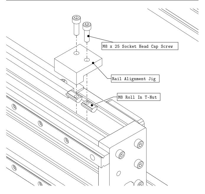
• Attach a Rail Adjustment Jig at one end of the gantry as indicated.
