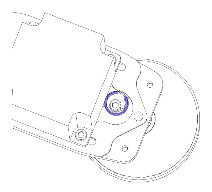
• Use a 16mm wrench to turn the Tensioner Cam against the motor.
