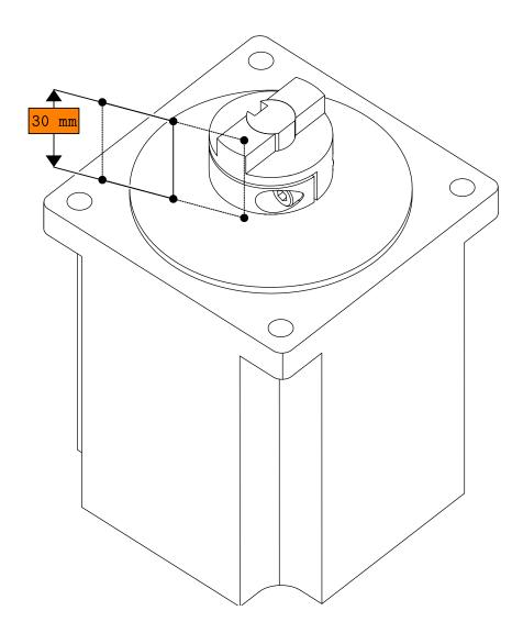
• Bring the upper face of the coupler flush with the end of the motor shaft.
