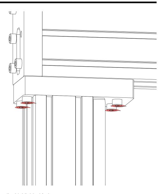
• Fully tighten the highlighted fasteners.
