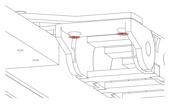
• Tighten the highlighted fasteners.
