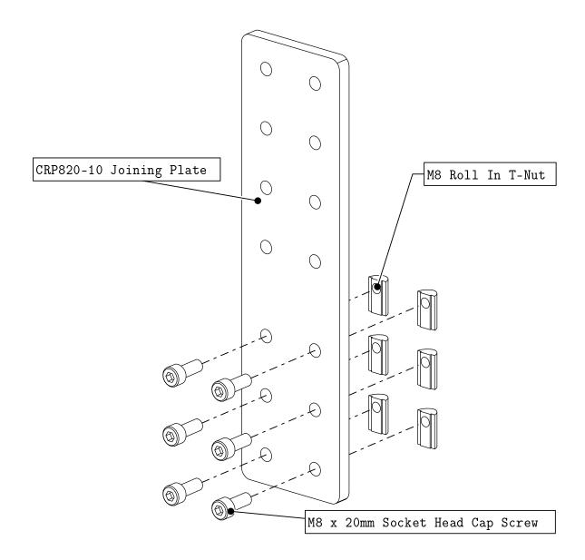
• Thread the indicated fasteners into the Riser Joining Plate.
