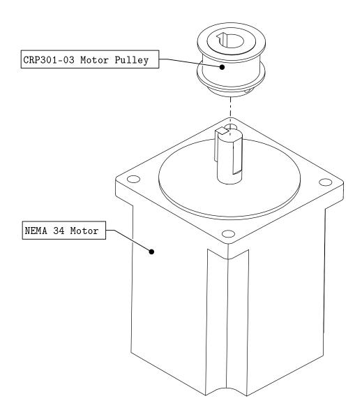
• Slide the motor pulley onto the motor shaft as indicated.
