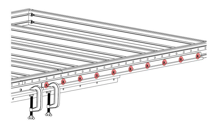
• Tighten the highlighted fasteners.
