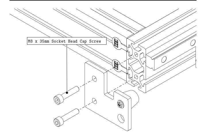
• Install a bumper to the extrusion as indicated.
