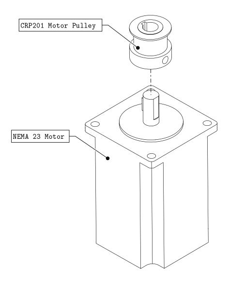
• Slide the motor pulley onto the motor shaft as indicated.
