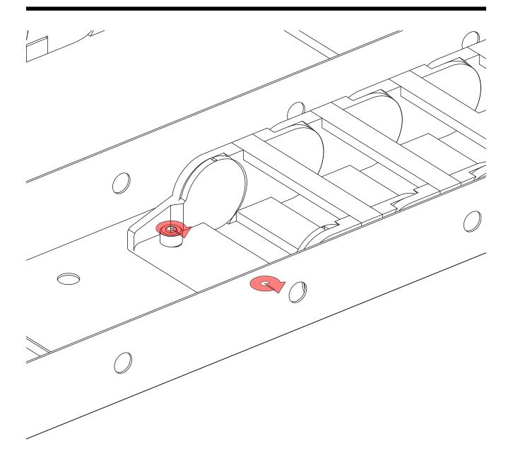
• Fully tighten the highlighted fasteners.
