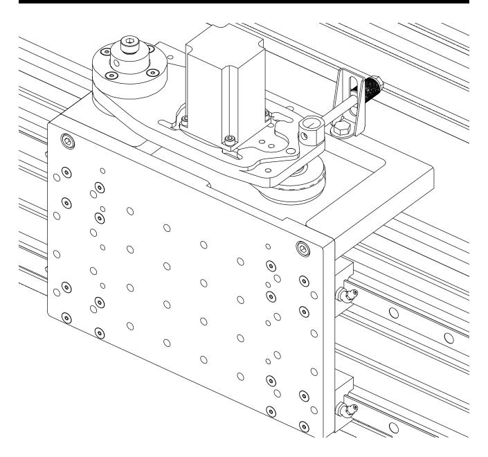
• The tensioner assembly should be installed as pictured.
