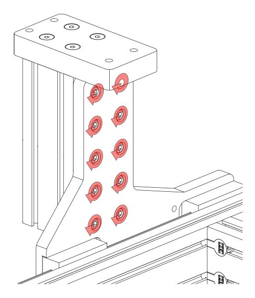
• Fully tighten the highlighted fasteners.
