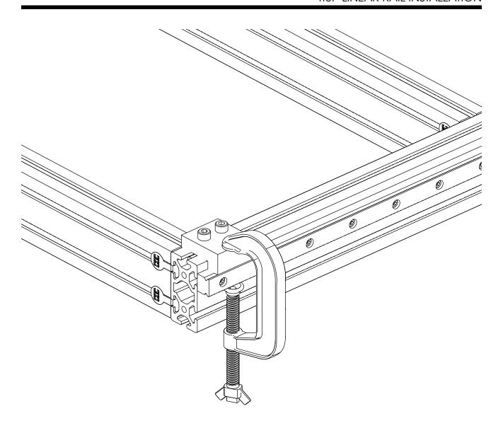
• Clamp the end of the linear rail to the jig.
