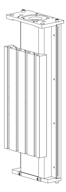
• Loosen the screws holding the dust covers to the Z-axis
