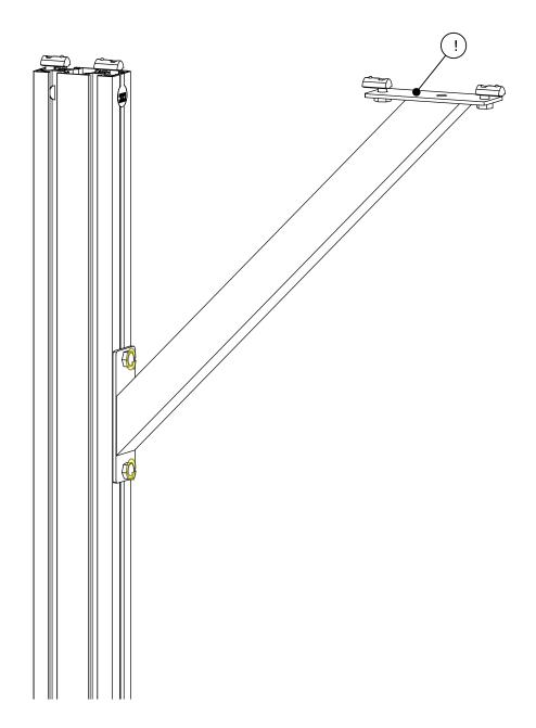
• Partially tighten the highlighted fasteners.
