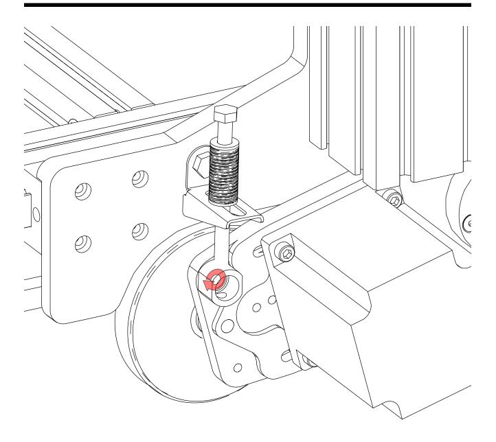
• Tighten the highlighted fasteners.
