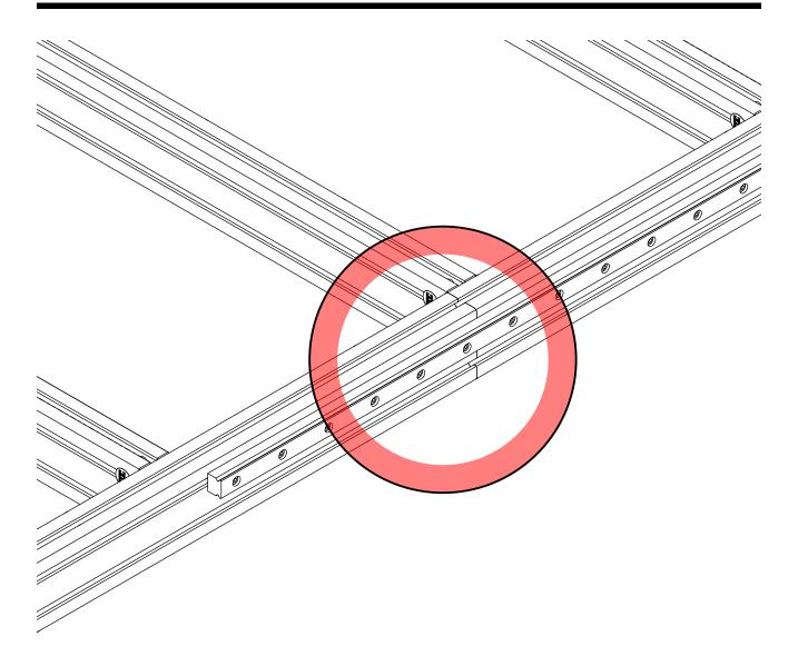
Note: The rail should cover the extrusion splice.
