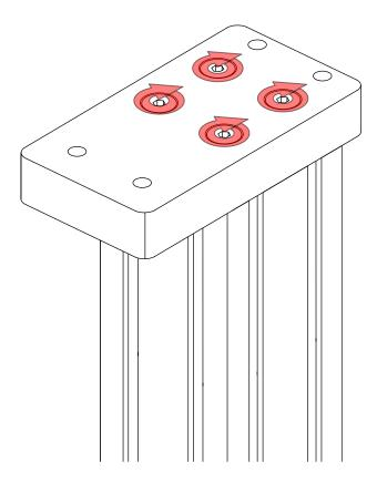
• Tighten the highlighted fasteners.
