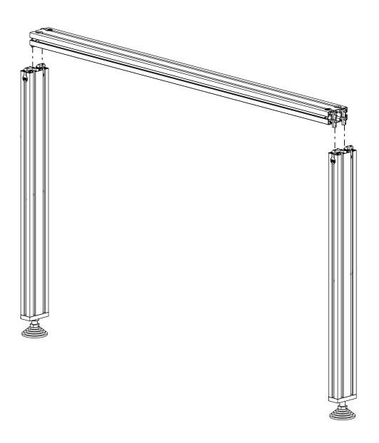
• Use a section of 1250mm Leg Extrusion to join two of the 750 mm Extrusion sections.
