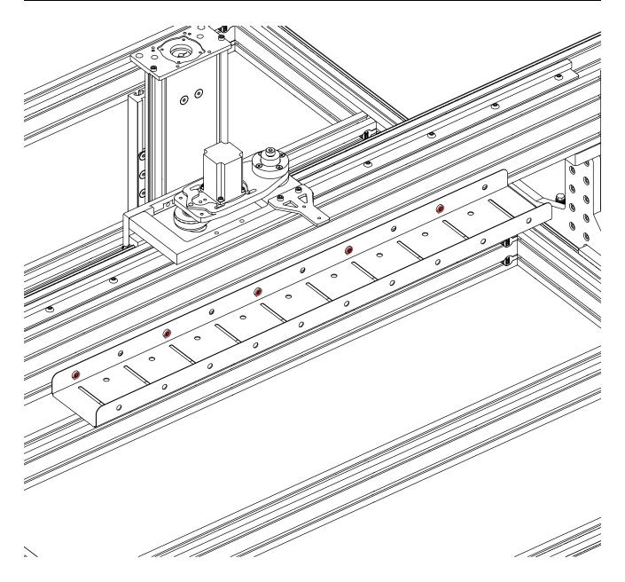
• Tighten the highlighted fasteners.
