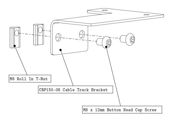
• Prethread fasteners into the riser cable track bracket as indicated.
