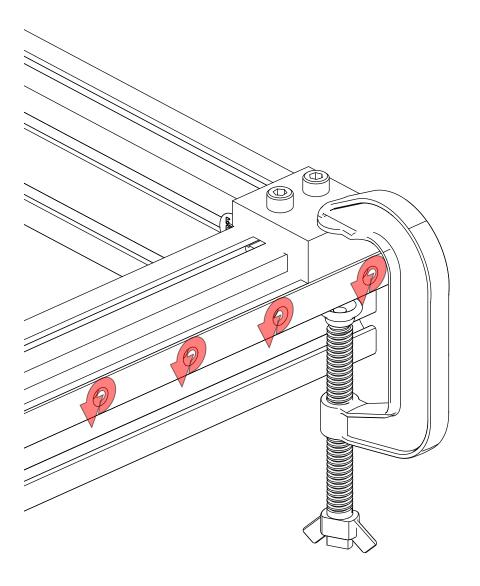
• Fully tighten fasteners of the clamped rail.
