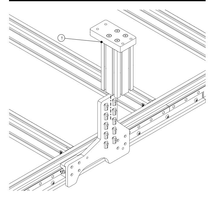
• Slide the extrusion assembly from the previous step onto the t-nuts on the riser plate.
