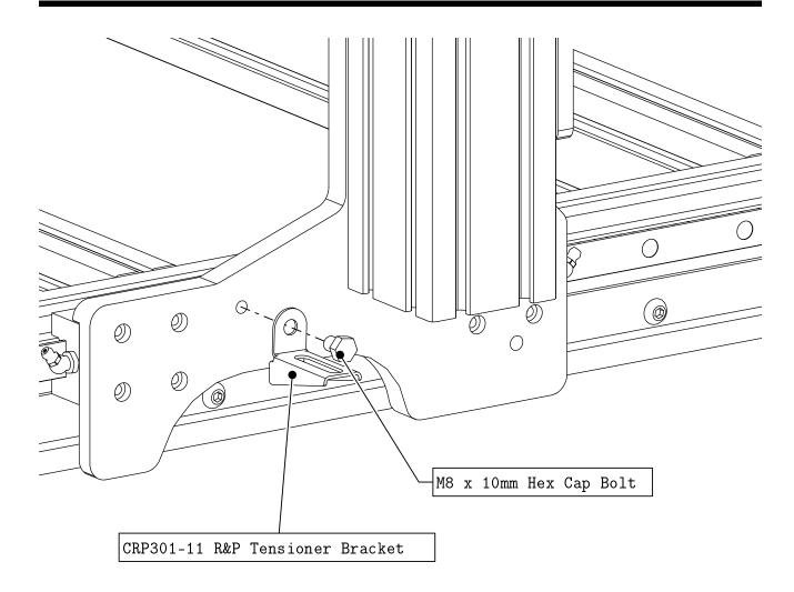
• Attach the Tension Bracket to the Riser Plate as indicated.
