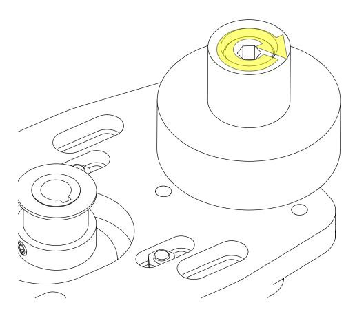
• Partially tighten the highlighted fastener.
