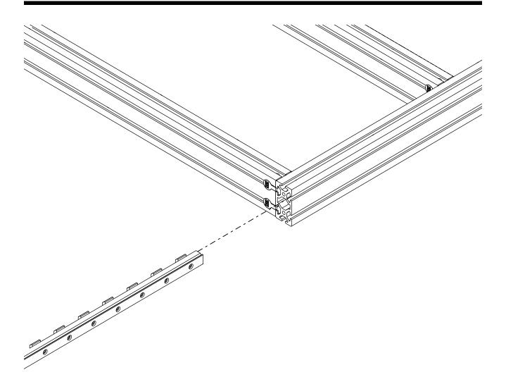
• Slide the shorter piece of rail into the extrusion.
