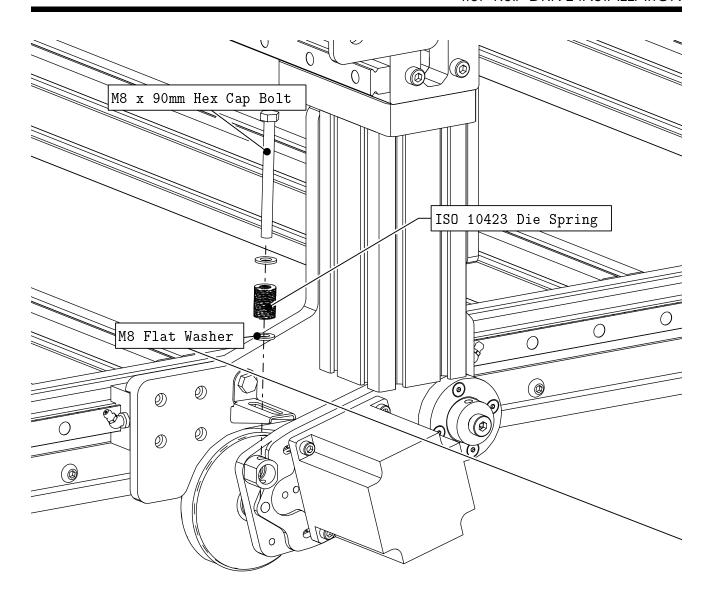
• Install the tension spring and bolt as indicated.
