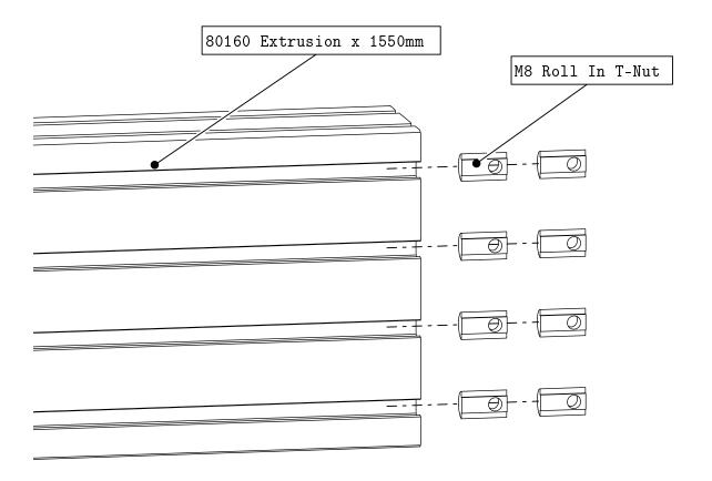
• Slide t-nuts into the indicated t-slots.
