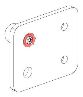
• Tighten the highlighted fastener.
