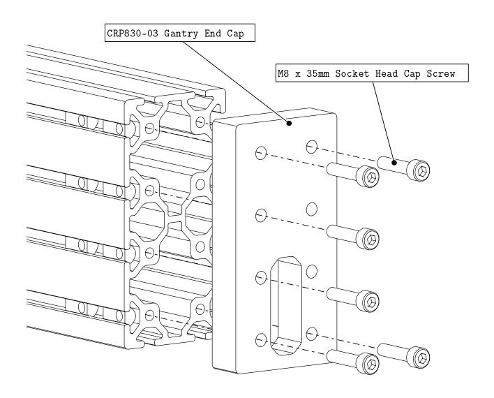
Install a Gantry End Cap on one end of the extrusion as indicated.
