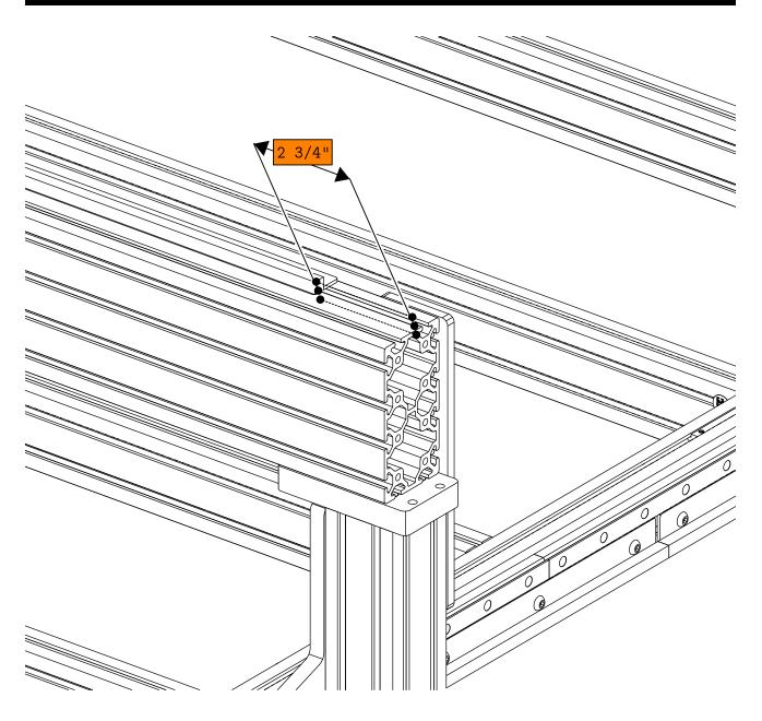
• Adjust the gear rack so that the end is approximatly 2 3/4" (70mm) from the end of the extrusion.
