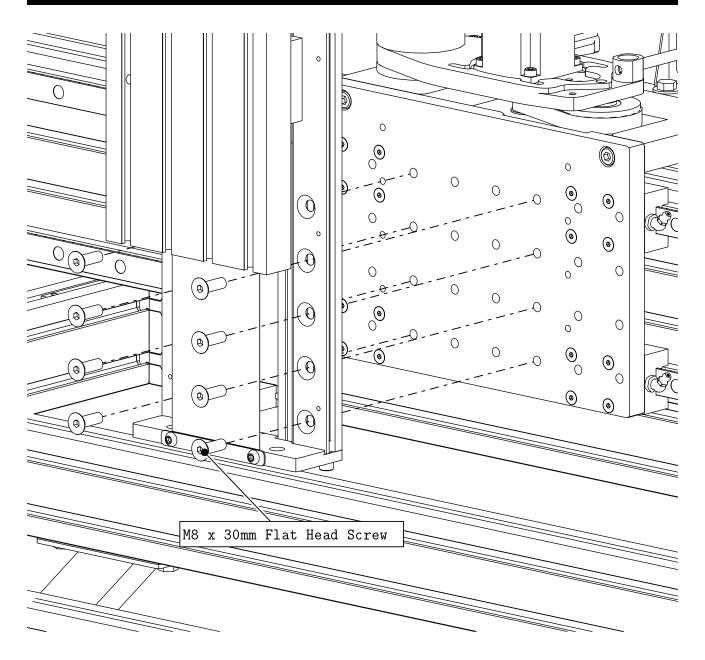
• Attach the Z-axis to the gantry carriage as indicated.
