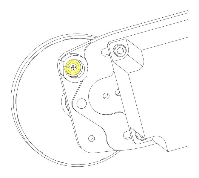
• Partially tighten the highlighted fastener.
