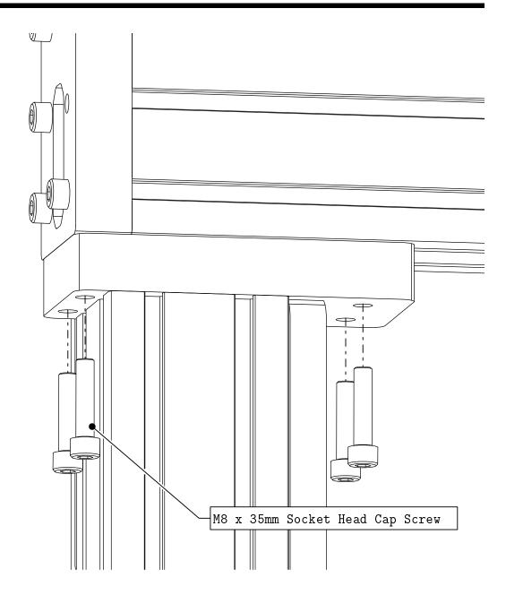
• Attach the gantry to the Interface Plate as indicated.
