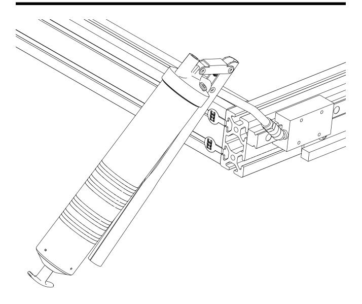
Note: The blocks will need to be relubricated periodically. The required interval will depend on machine use, loads, and ambient conditions. We suggest evaluating each month by cleaning your linear rails, moving the blocks along them, and checking for a lubricant film. If a film is not present, then add one additional pump of grease to your blocks.
