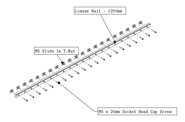
• Thread fasteners into the linear rail as indicated.
