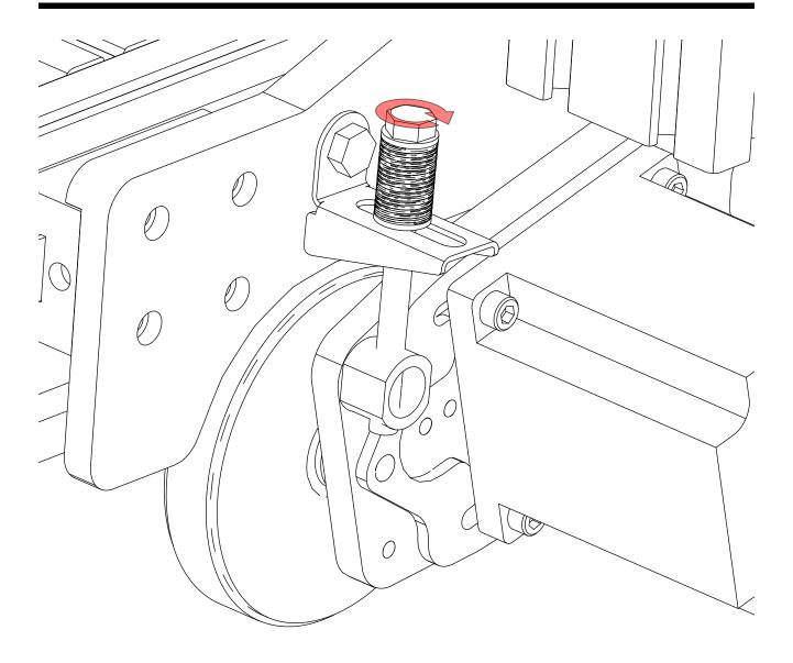
• Adjust the tensioner bolt until gear is seated in rack, then tighten another 3 revolutions.
