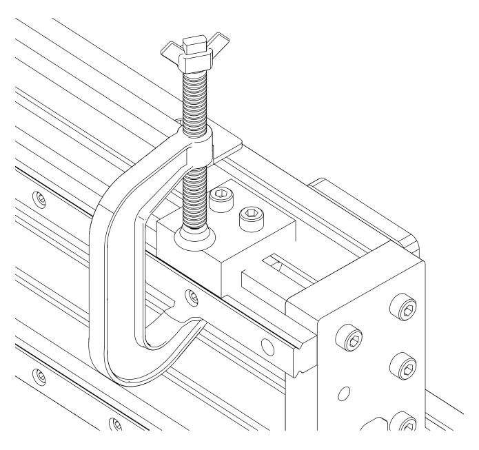
• Clamp the end of the rail to the rail Rail Adjustment Jig.
