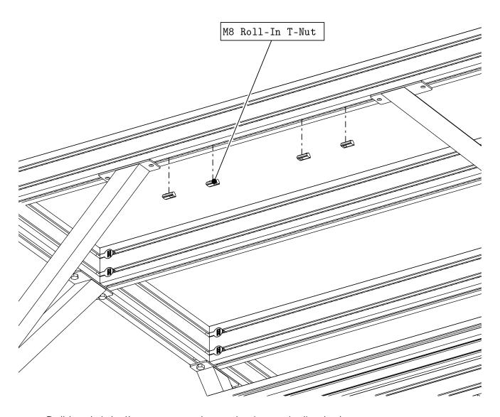
• Roll t-nuts into the crossmember extrusion as indicated.
