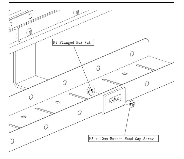
• Adjust the other bracket as necessary and attach to the cable tray as indicated.
