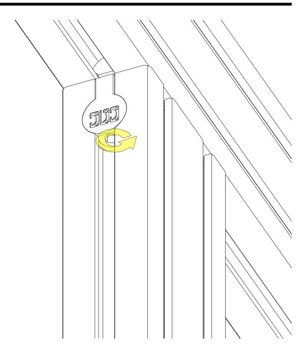
• Partially tighten the highlighted fasteners.
