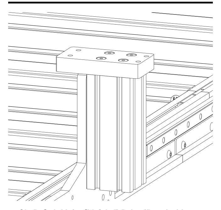
• Bring the Gantry Interface Plate flush with the top of the gantry plate
