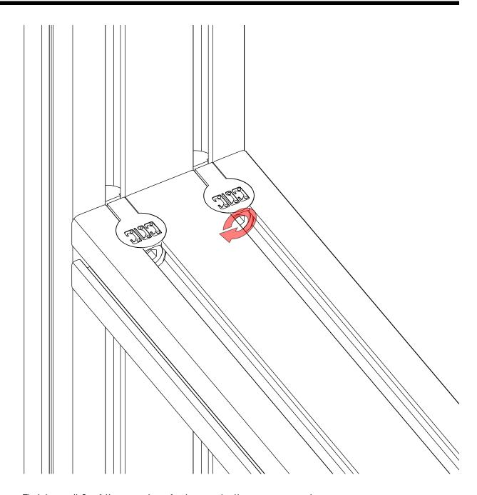
• Tighten all 8 of the anchor fasteners in the crossmember.
