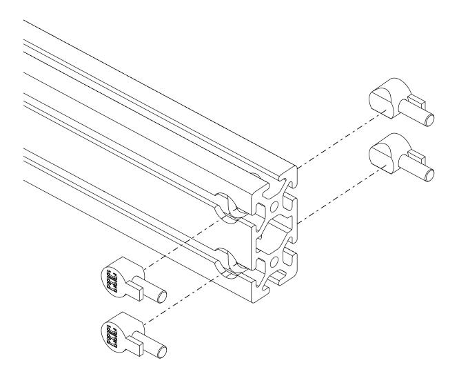
• Slide the anchor assembly into the extrusion.
