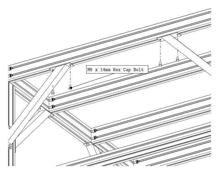
• Fasten the gusset to the extrusion as indicated.
