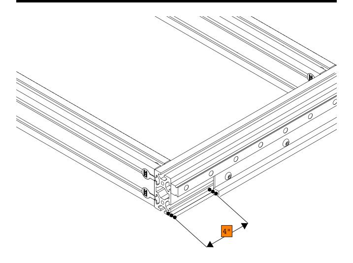
• Ensure the gear rack is spaced 4" (100mm) from the end of the extrusion as pictured.
