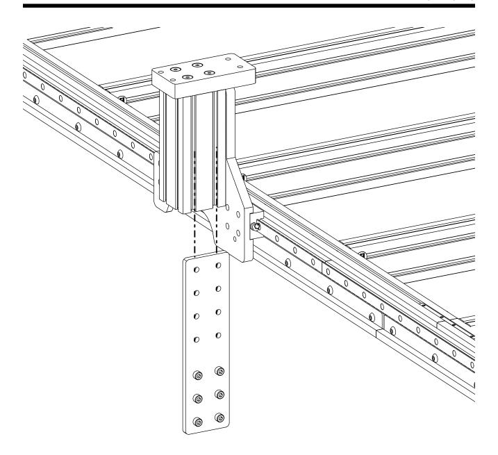
• Slide the Joining Plate into the indicated t-slots.
