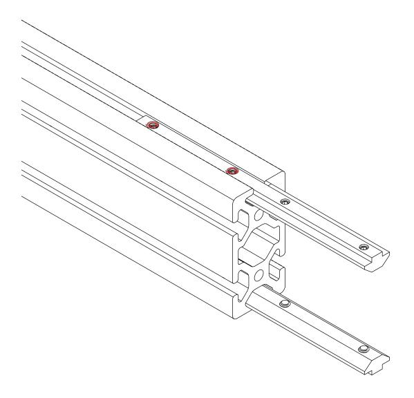
• Tighten the highlighted fasteners.
