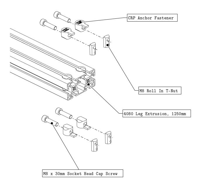
• Thread the socket head cap screws into the t-nuts through the anchor fasteners as indicated.
