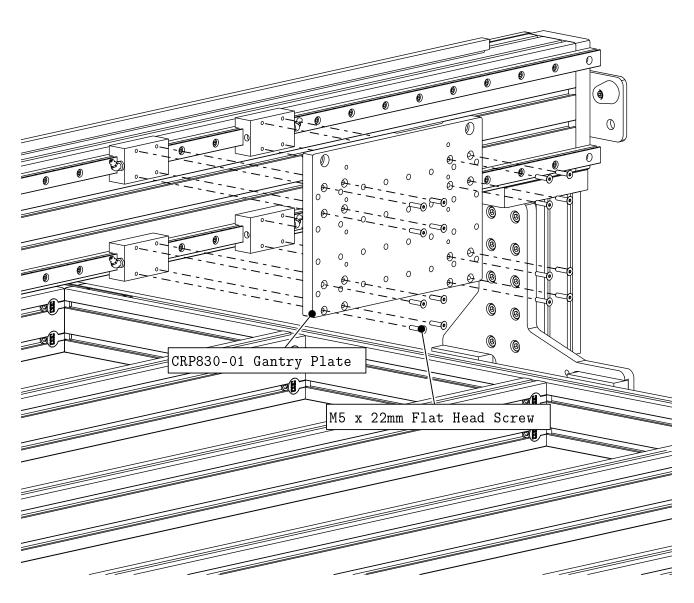
• Attach the Gantry Plate to the bearing blocks as indicated.
