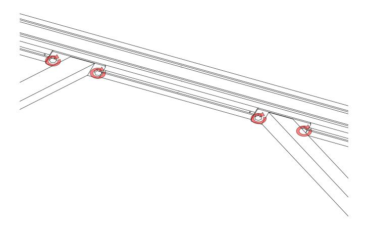
• Tighten the highlighted fasteners.
