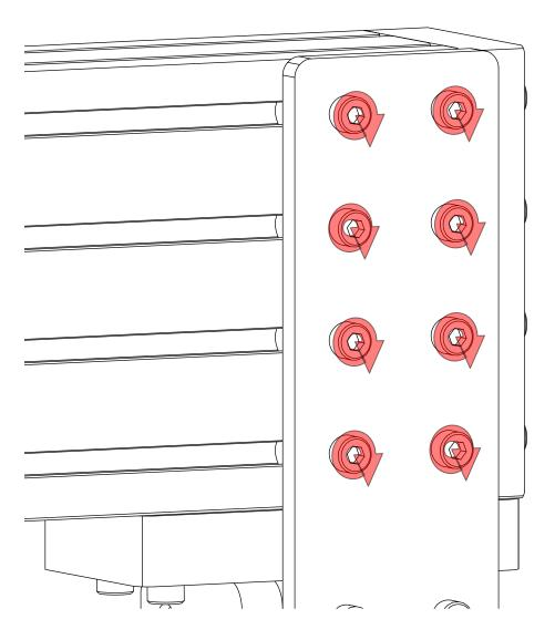
• Tighten the highlighted fasteners.
