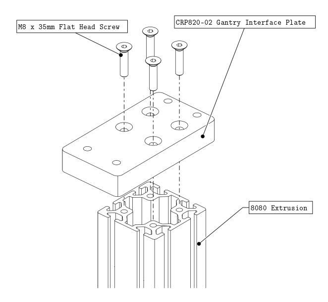
• Install a CRP820-02 Gantry Interface Plate to a piece of 8080 extrusion as indicated.
