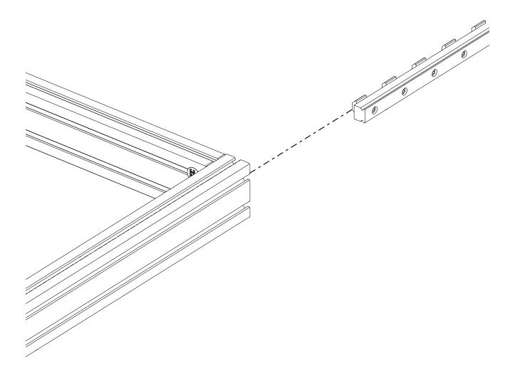
• Slide one of the 1600mm rails into the extrusion t-slot as indicated.
