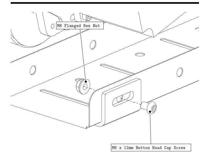
• Attach the cable track to the front bracket.
