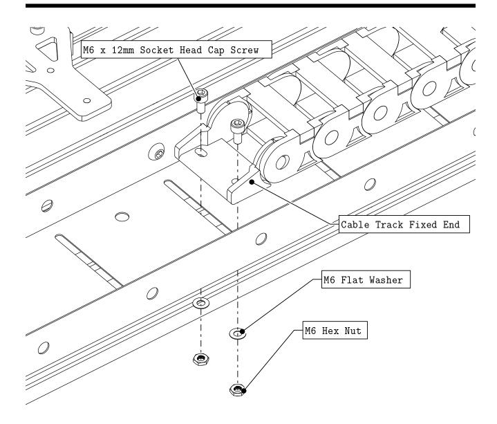
• Attach the fixed end of the cable track to the tray as indicated.
