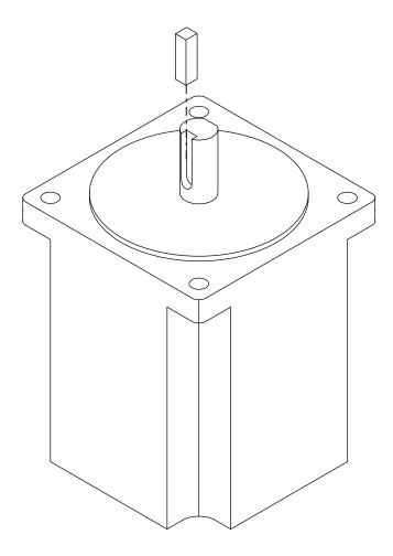
• Using a pair of pliers, remove the key from your remaining motor.
