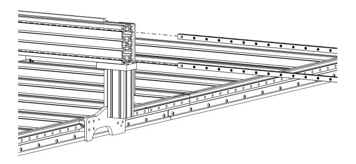
• Slide the threaded rails into the indicated t-slots.
