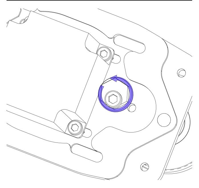
• Use a 16mm wrench to turn the Tensioner Cam against the motor.
