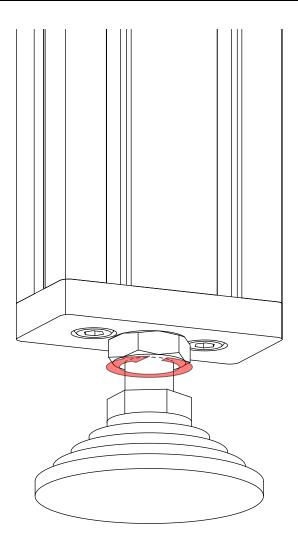
• Fully tighten the highlighted fasteners.
