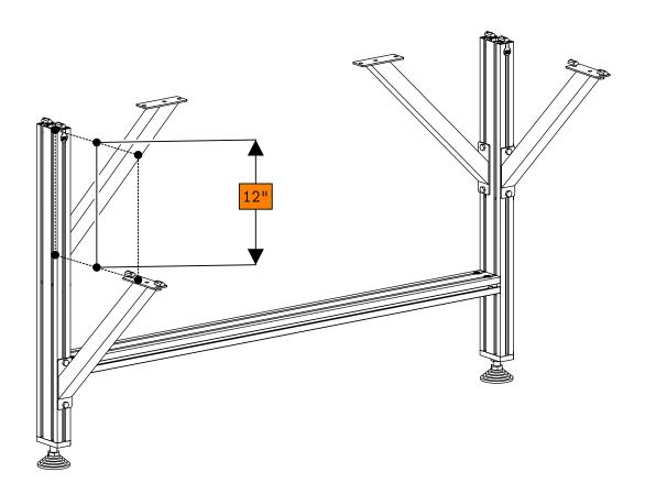
• Install 3 additional gussets to the leg assembly as indicated.
