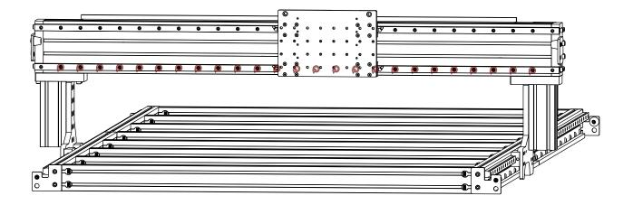
• Fully tighten the highlighted fasteners.
