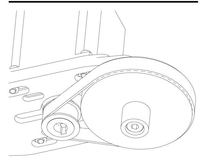
• Hold the Tensioner Cam against the motor to generate belt tension.
