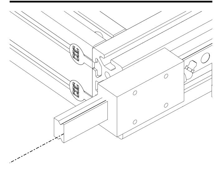
• Use the rail to push the plastic bearing retainer out of the block as indicated.
