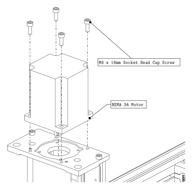
• Install the z-axis motor as indicated.
