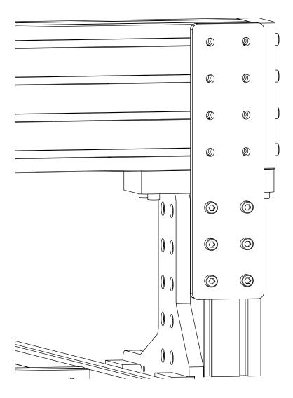
• Align the t-nuts in the gantry with the holes on the Joining Plate.
