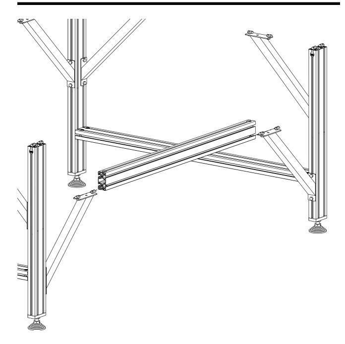
• Slide the 1080mm length of leg extrusion onto the lowered gussets as indicated.
