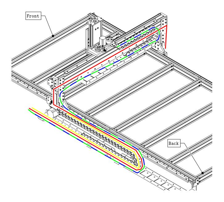
The colored lines indicate the recommended routing for motor cables in the system:
