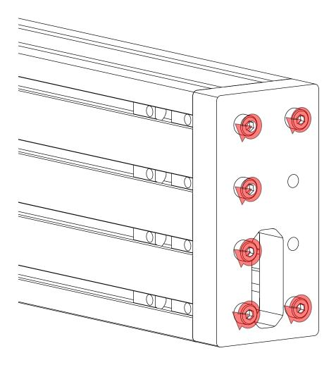
• Tighten the highlighted fasteners.
