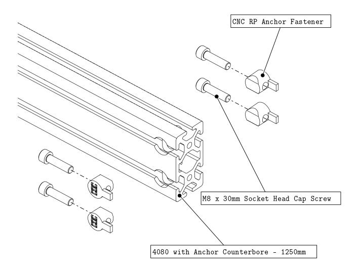
• Thread the socket head cap screws into the anchor fasteners as indicated.
