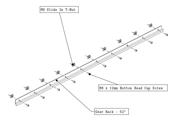
• Thread fasteners into the gear rack as indicated.
