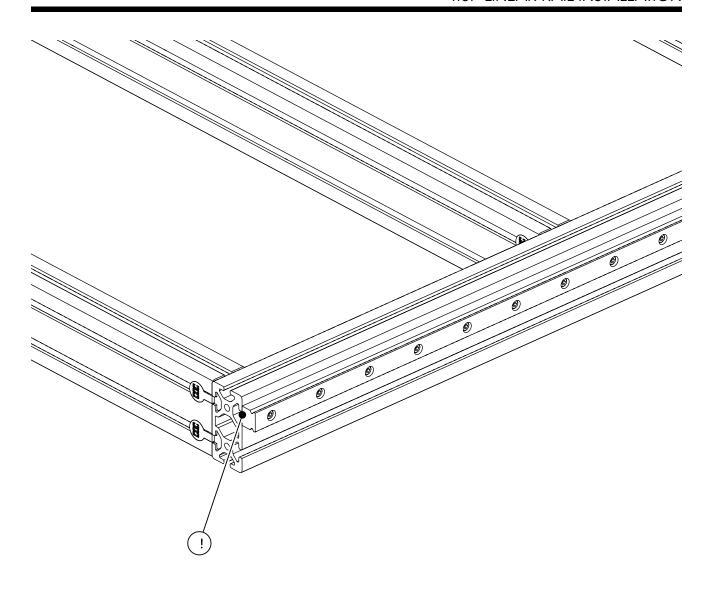
Note: The rail should be roughly flush with the end of the extrusion.
