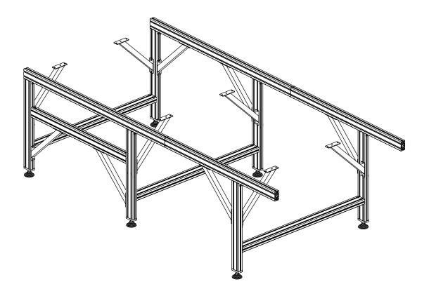
• Use the remaining splice kits to install a 1250mm section of extrusion of the other side of the frame.
