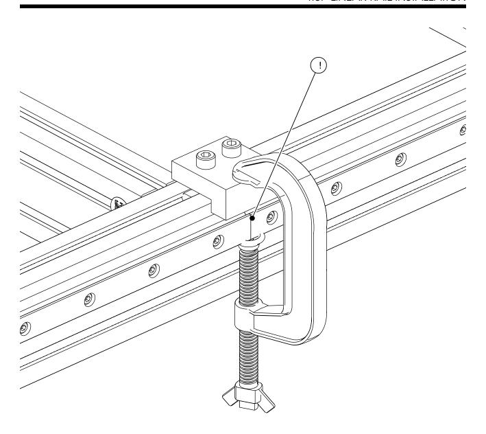
• Ensure the rails are flush at the splice.
