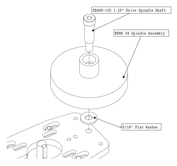
• Attach the drive spindle to the R&P Plate as indicated.
