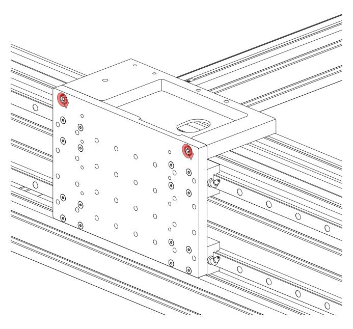
• Tighten the highlighted fasteners.
