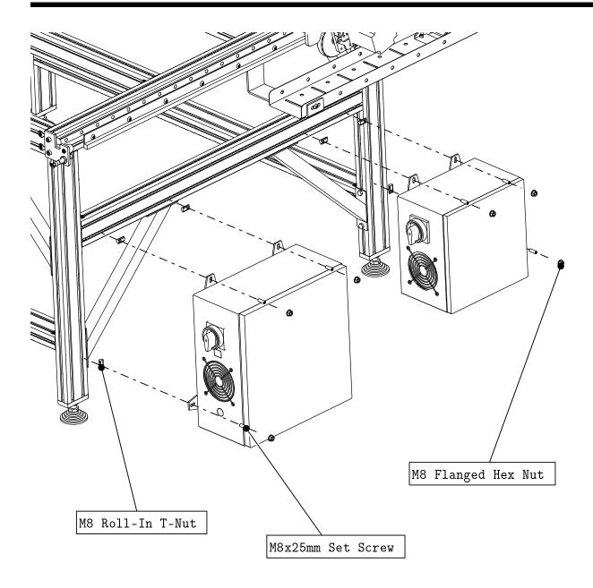
If you purchased a Plug and Play Electronics Kit and/or a VFD, you may attach these to the leg kit using the indicated fasteners.
