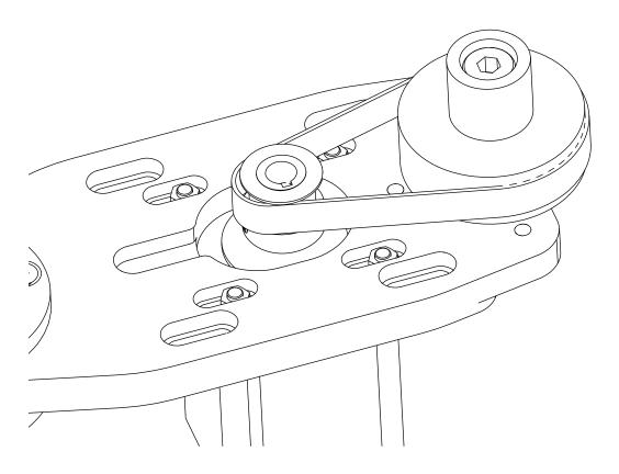
• Slide the motor closer to the drive spindle if necessary.
