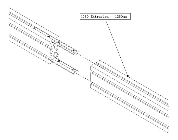
• Slide a 1250mm section of extrusion onto the splice bars.
