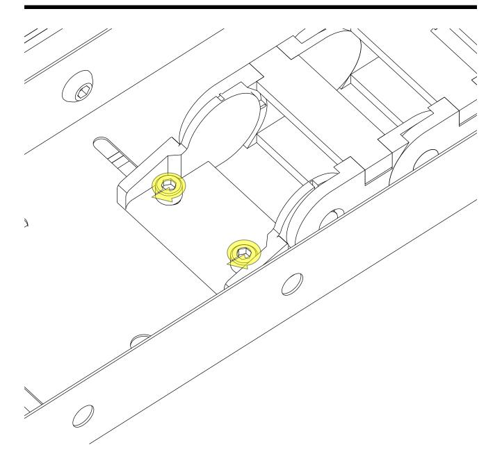
• Partially tighten the highlighted fasteners.
