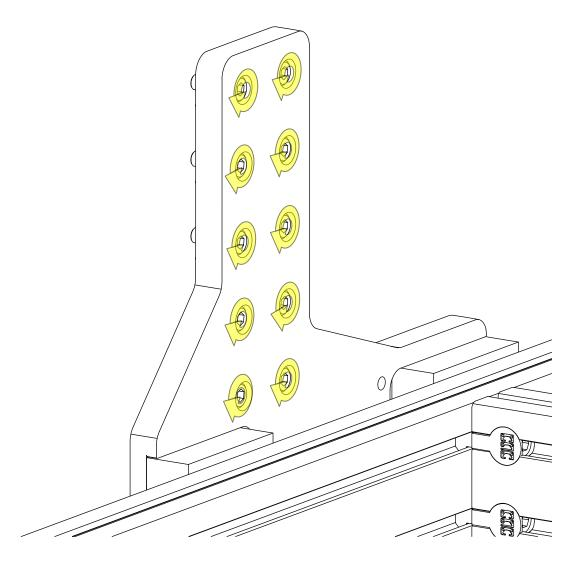
• Partially tighten the highlighted fasteners.
