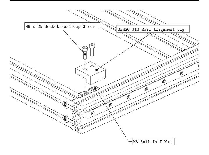
• Attach the rail alignment jig to the extrusion as indicated.
