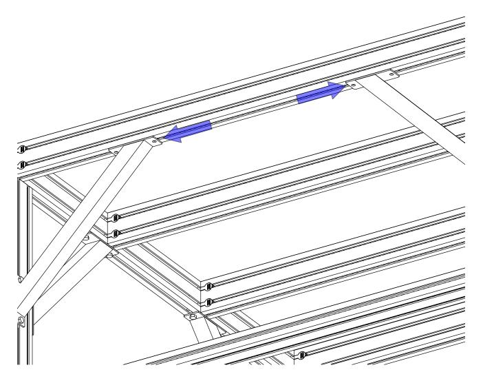
• Slide the t-nuts under the holes of the gusset.
