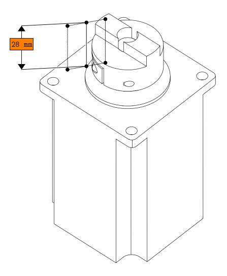
• Bring the lower face of the coupler flush with the end of the motor shaft.
