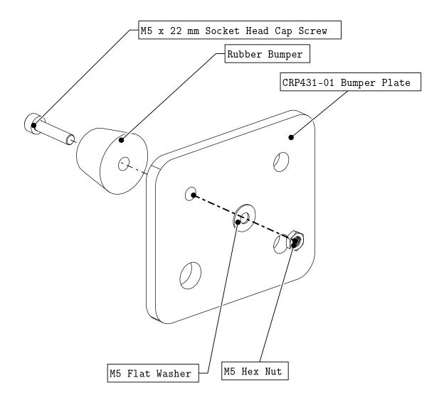
• Attach the rubber bumper to the gantry bumper plate.
