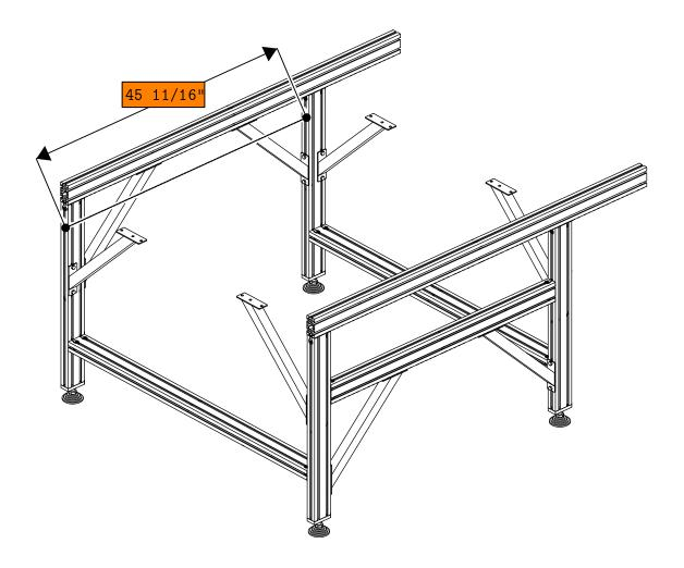
• Position the leg assemblies 45 11/16" (1160mm) from the front of the machine as indicated.
