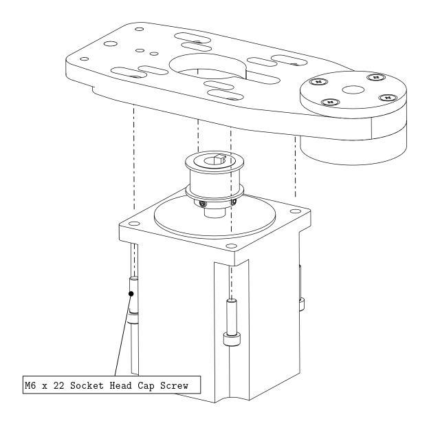
• Attach the motor to the R&P Plate as indicated.
