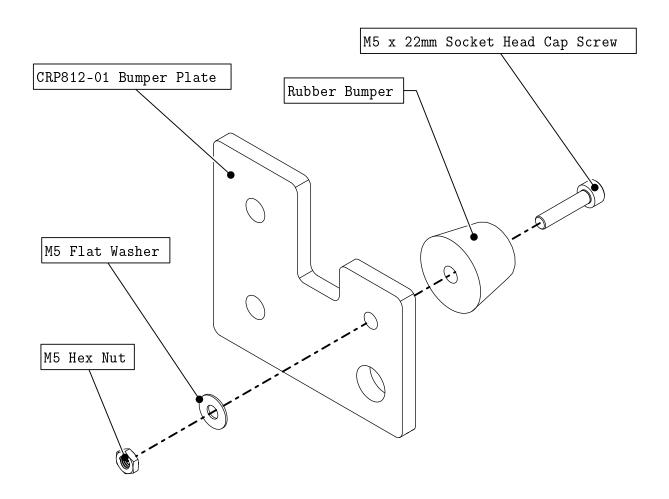
• Attach the rubber bumper to the bumper plate as indicated.
