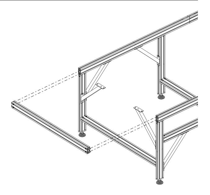
• Slide the t-nuts into the frame extrusion as indicated.
