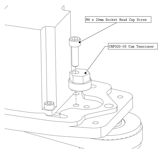
• Attach the Tensioner Cam to the R&P Plate as indicated.
