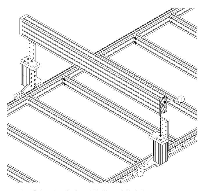
• Carefully lower the extrusion onto the risers as indicated.
