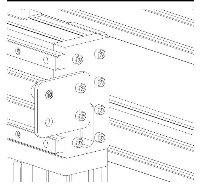
• Tighten the highlighted fasteners.
