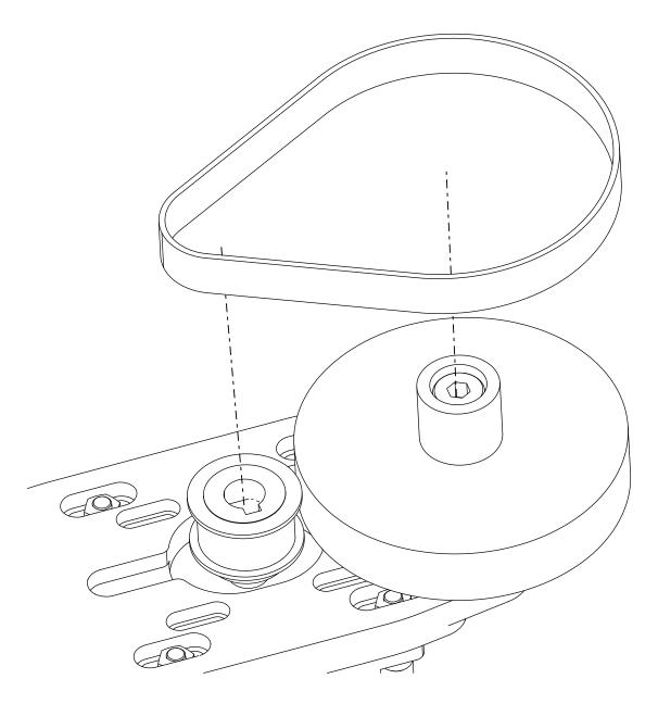
• Slide the drive belt around the motor pulley and drive spindle.
