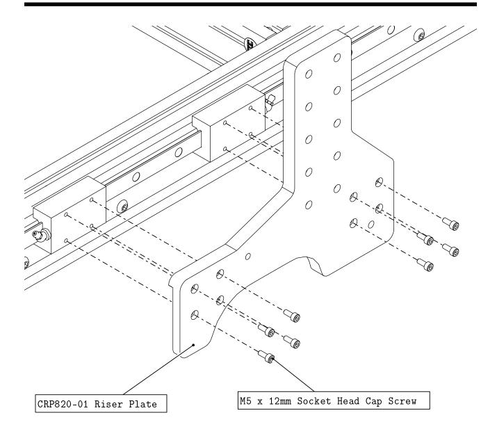
• Install a riser onto the linear bearing blocks as indicated.
