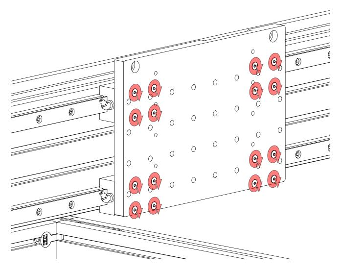
• Tighten the highlighted fasteners.
