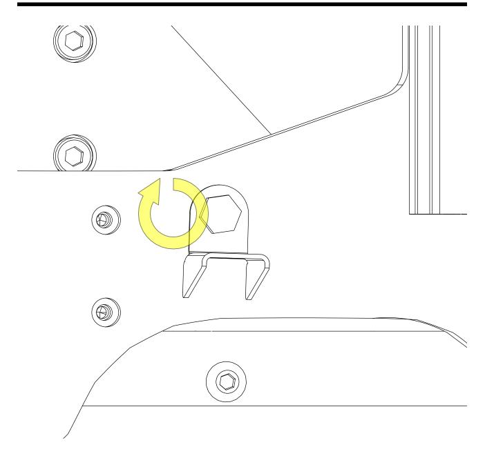
• Partially tighten the highlighted fastener.
