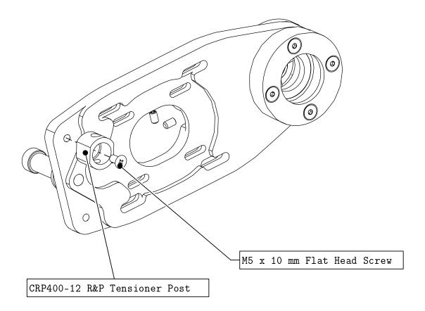
• Attach the Tension Post to the R&P Plate as indicated.
