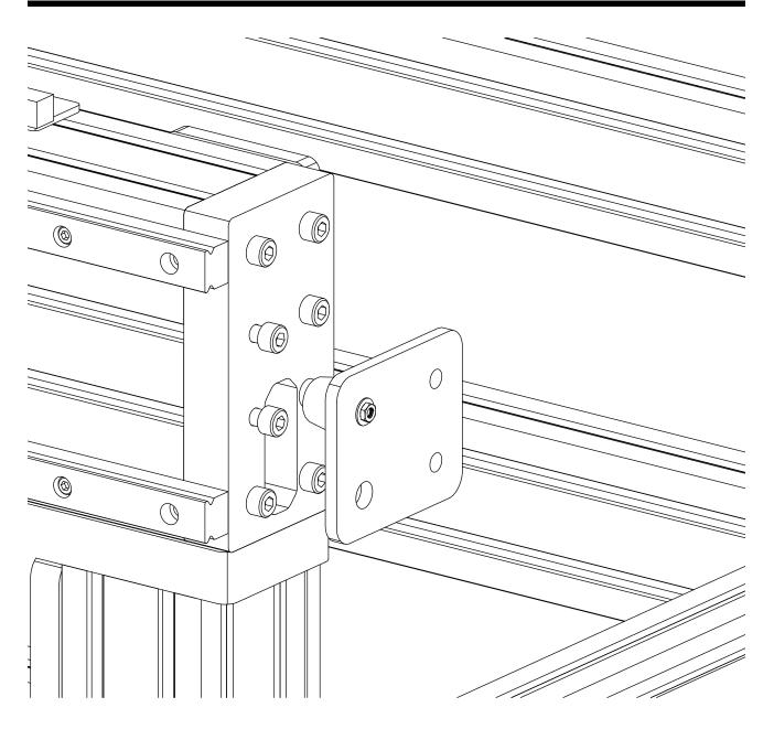
• Attach the bumper plate to the gantry end cap as indicated.
