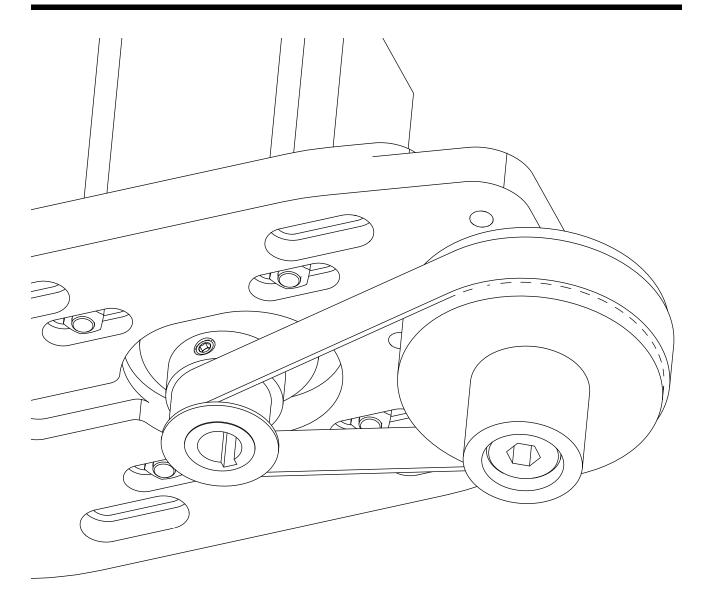
• Hold the Tensioner Cam against the motor to generate belt tension.
