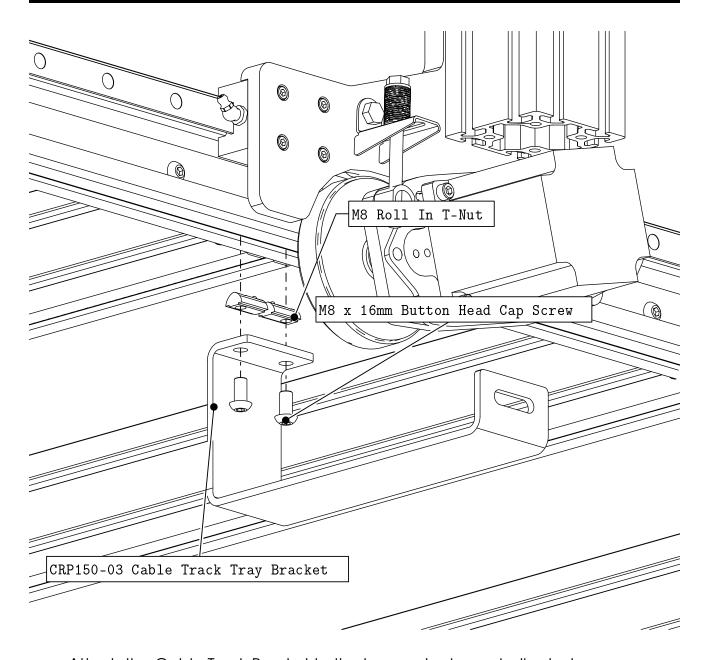
• Attach the Cable Track Bracket to the base extrusion as indicated.
