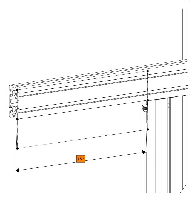
$\bullet\,$  Position the leg kit 16.15" (410mm) from the end of the extrusion as indicated.
