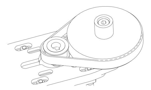
• Slide the motor closer to the drive spindle if necessary.
