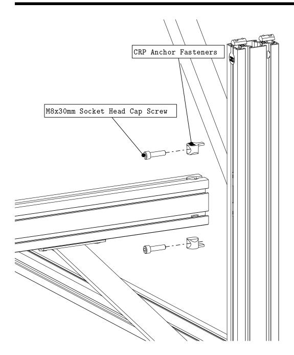
• Install anchor fasteners as indicated.
