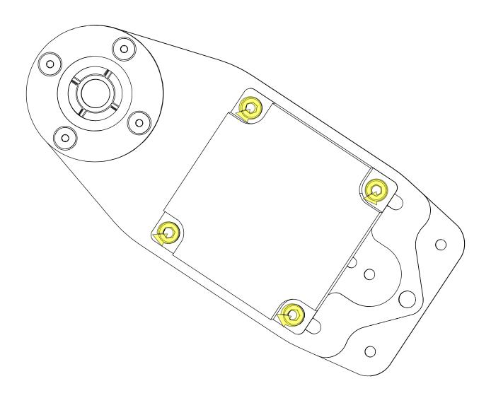
• Partially tighten the highlighted fasteners.
