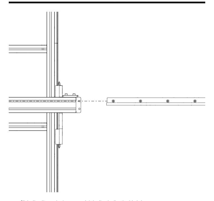
• Slide the threaded gear rack into the indicated t-slot.
