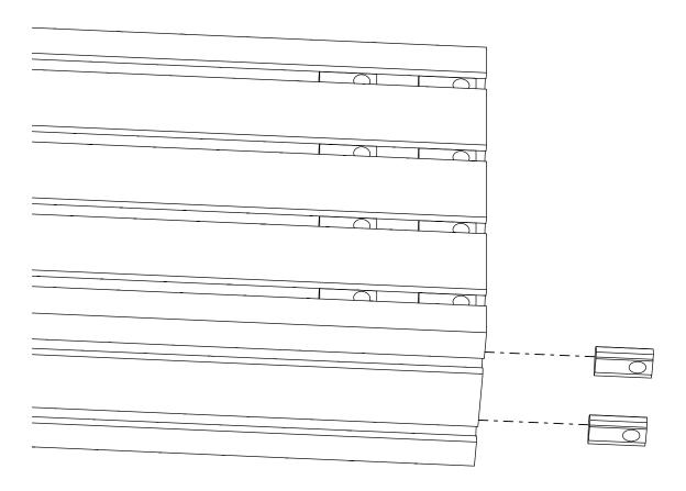
• Slide t-nuts into the indicated t-slots.
