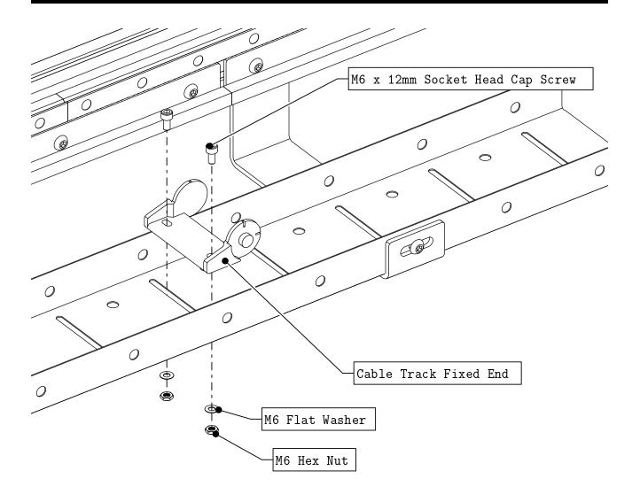
• Attach the fixed end of the cable track to the tray, 5 slots from the end of the tray as indicated.
