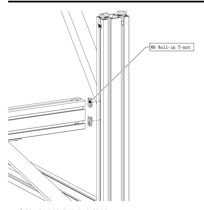
• Roll two t-nuts into the indicated t-slot.
