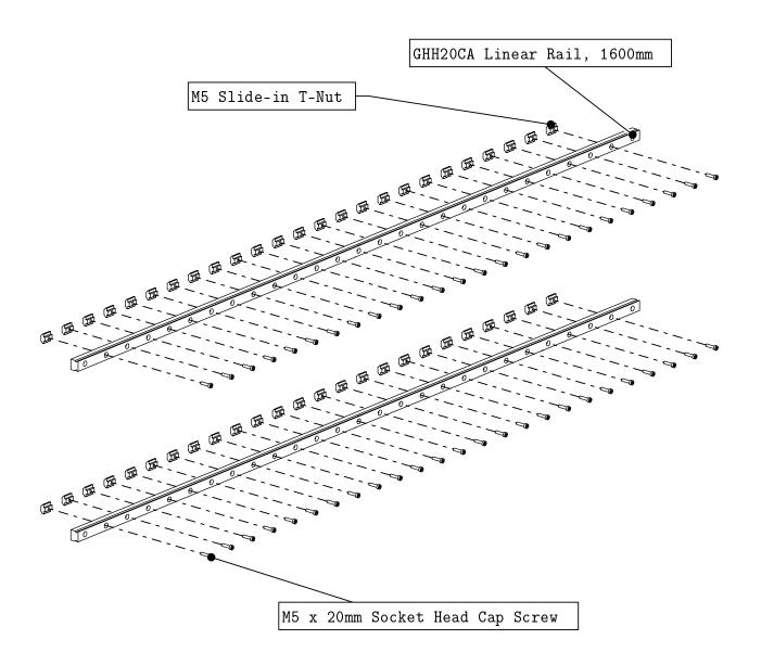
• Thread the indicated fasteners into the linear rails.
