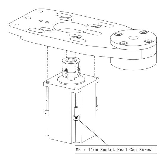
• Attach the motor to the R&P Plate as indicated.
