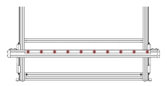
• Tighten the highlighted fasteners.
