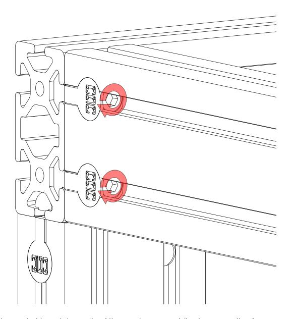
• Tighten the socket heads in each of the anchor assemblies to secure the frame.
