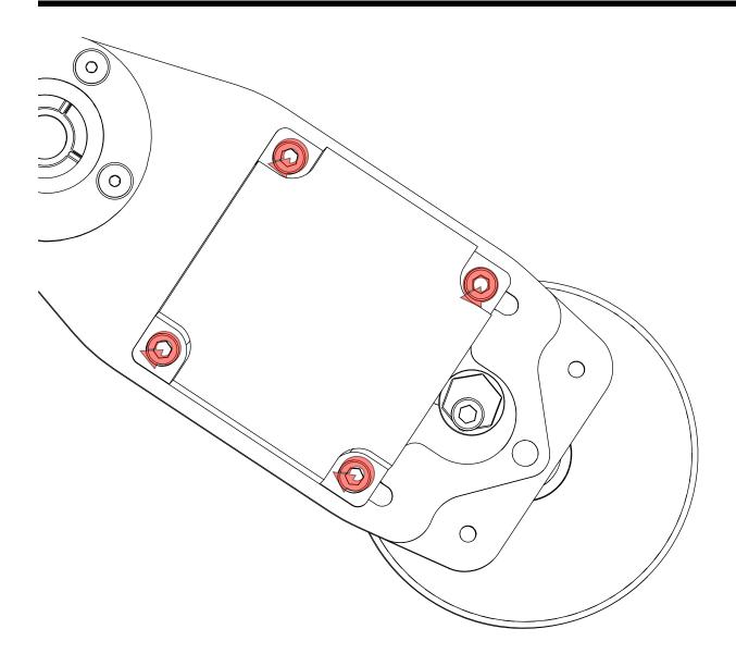
• Fully tighten the highlighted fasteners.
