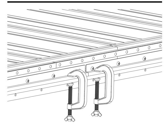
• Clamp an additional section of gear rack to the two sections to align the gear rack teeth.
