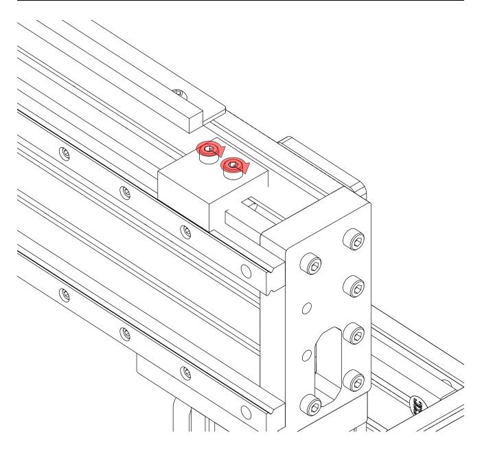
• Tighten the highlighted fasteners.
