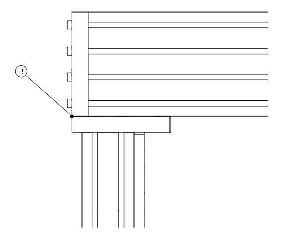
• Bring the End Cap flush with the Interface Plate as indicated.
