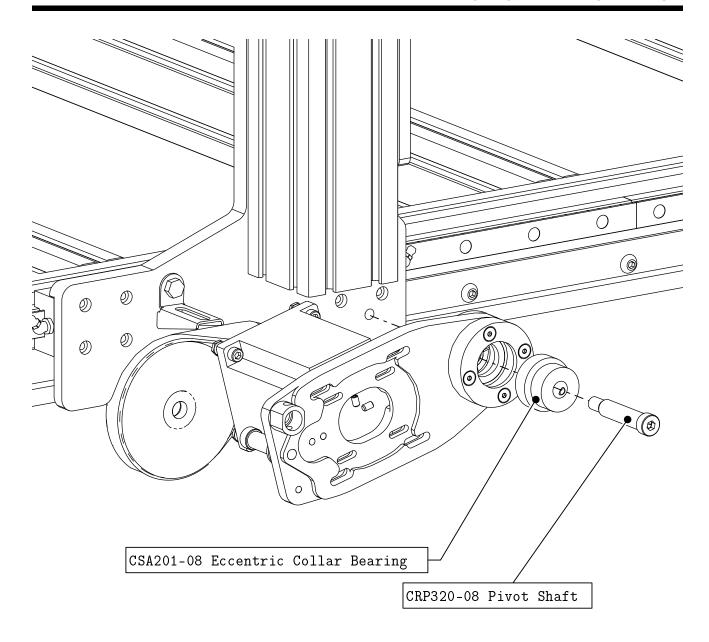
• Attach the R&P Assembly to the Riser Plate as indicated.
