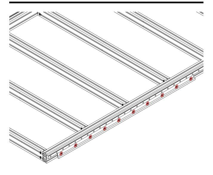
• Tighten the indicated fasteners.
