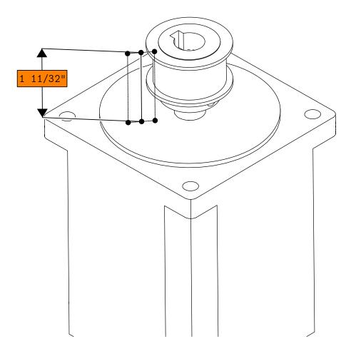
• Adjust the motor pulley such that the top of the pulley is 1 11/32" (34mm) from the motor flat.
