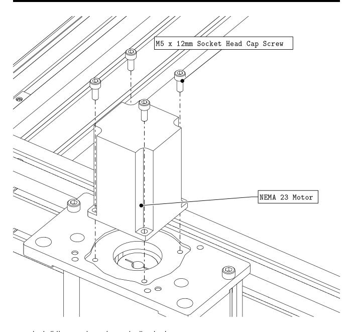
• Install the z-axis motor as indicated.
