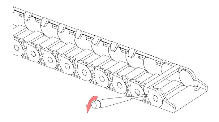
• Use a screwdriver to lift open the cable track sections, and route the cable through the track.
