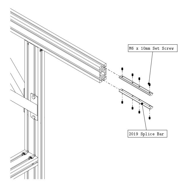
• Install two spice bars into the end of the frame extrusion as indicated.
