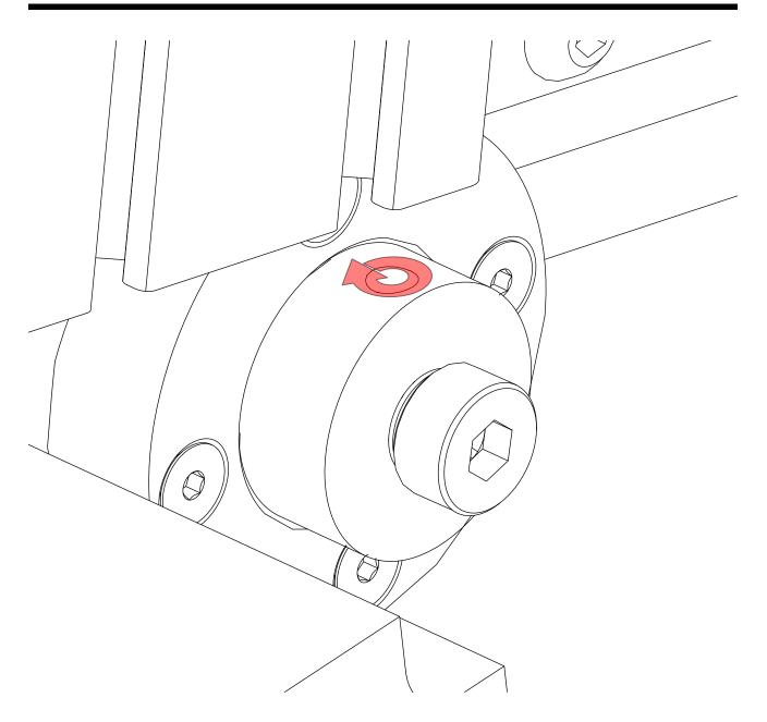
• Tighten the set screw on the side of the eccentric.
