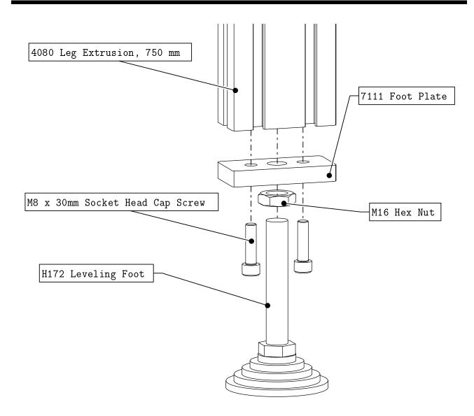
• Install a foot assembly onto a piece of 750mm Leg extrusion as indicated.
