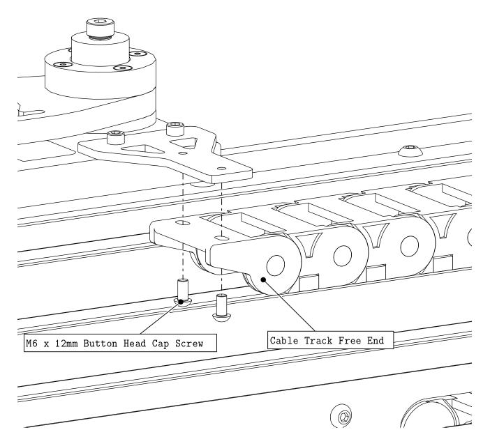
• Attach the remaining end of the cable track to the bracket as indicated.
