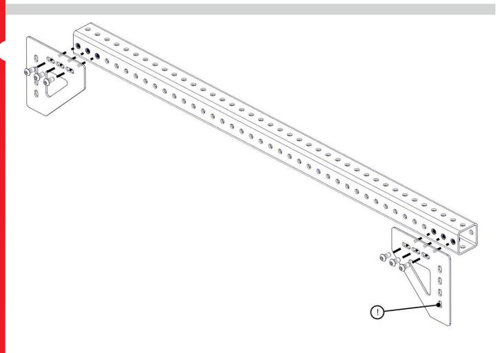
Loosely attach the CRP113-07 Corner Brackets to the remaining tubes. \\
