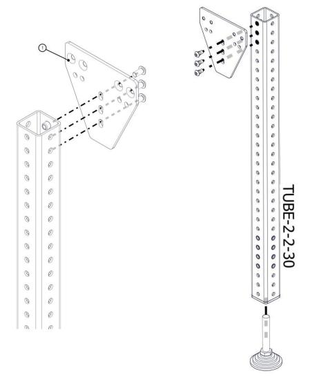
Attach the CRP113-09 Machine Connection Bracket to the top of the 30" steel tubes as shown. Thread the M16 Leveling Feet into the bottom of the tube.
