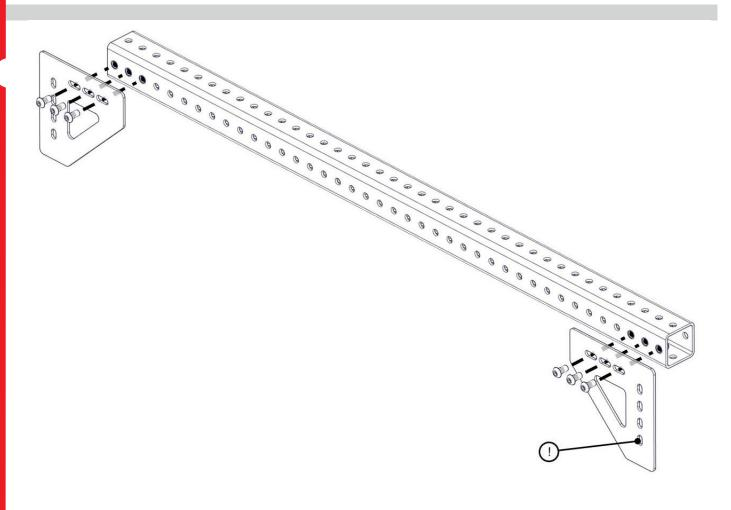
Loosely attach the CRP113-07 Corner Brackets to the remaining tubes. Ensure the sides of the brackets with 4 slots are vertical.
