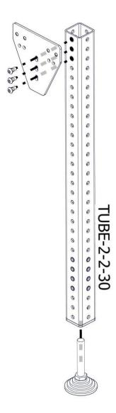
Attach the CRP113-09 Machine Connection Bracket to the top of the 30" steel tubes as shown. Thread the M16 Leveling Feet into the bottom of the tube.
